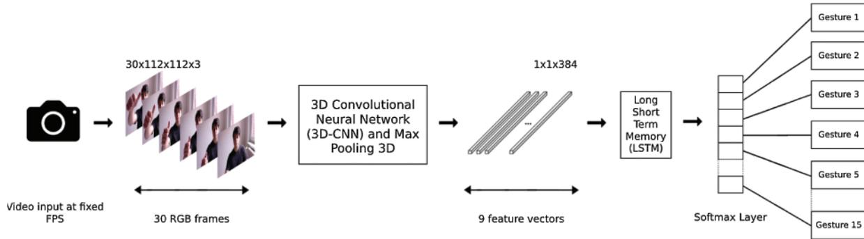
**Figure 3:** The proposed model pipeline
