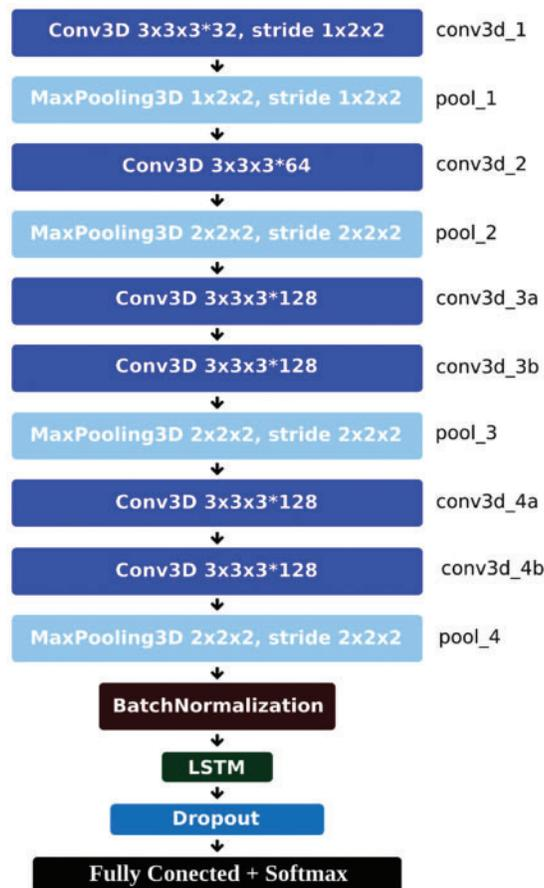
Figure 6: The proposed 3D-CNN + LSTM architecture
