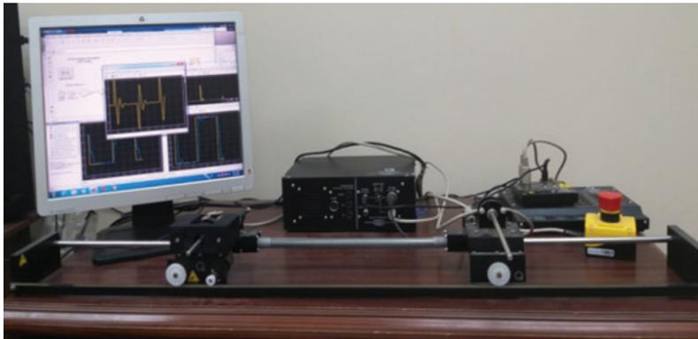
**Figure 5:** Experimental setup for linear flexible joint cart system
