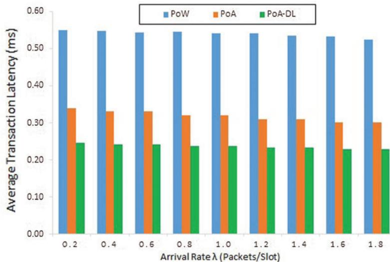
**Figure 4:** Average transaction latency for both PoA and PoW-based blockchain systems
