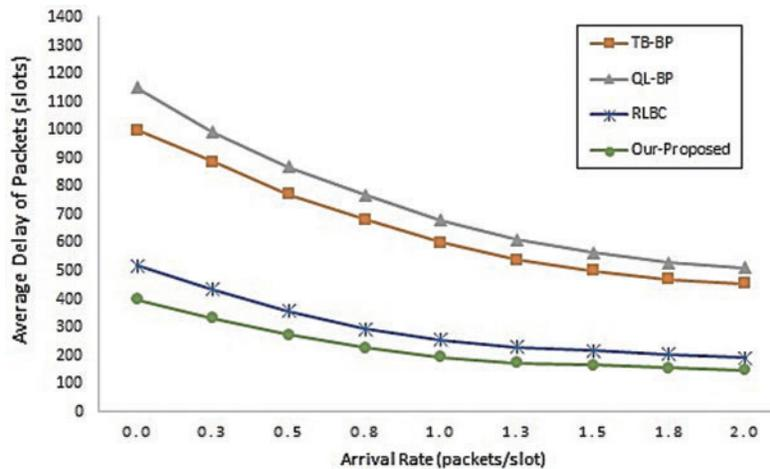
**Figure 3:** Average delay of packets with 50% malicious nodes
