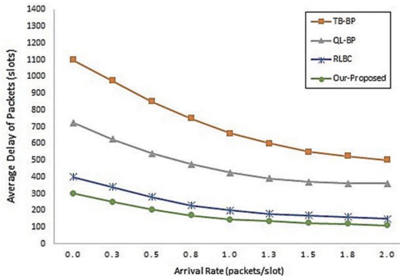
Figure 2: Average delay of packets with 25% malicious nodes
