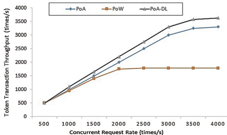
**Figure 5:** Throughput of transaction token for both PoA-DL, PoA and PoW-based blockchain systems
