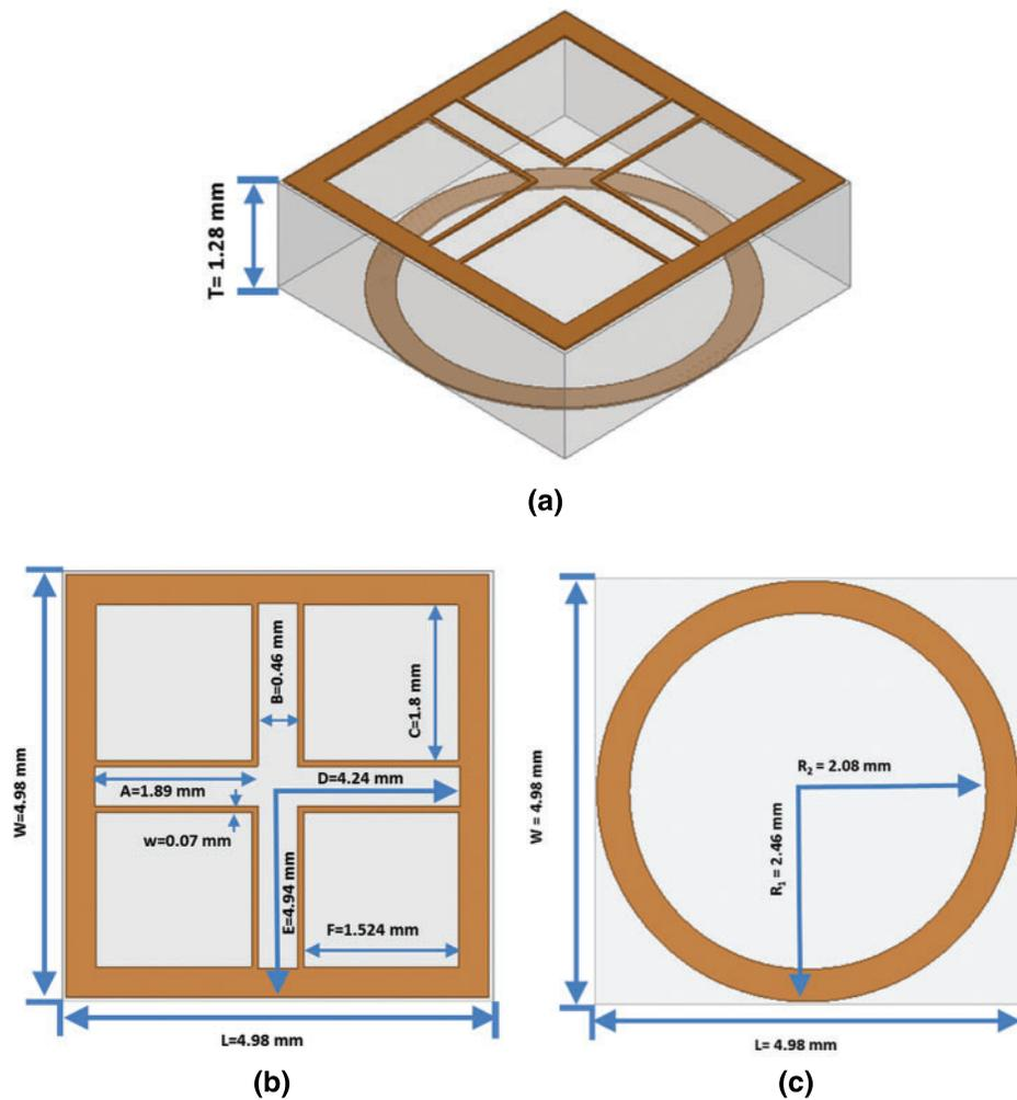
**Figure 1:** Geometry of dual layer UWB FSS, (a) 3D-view of UWB FSS unit cell, (b) upper view of square loop element, (c) bottom view of circular loop element
