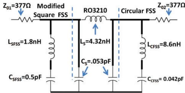
Figure 2: Equivalent circuit model (ECM) of the proposed UWB FSS
