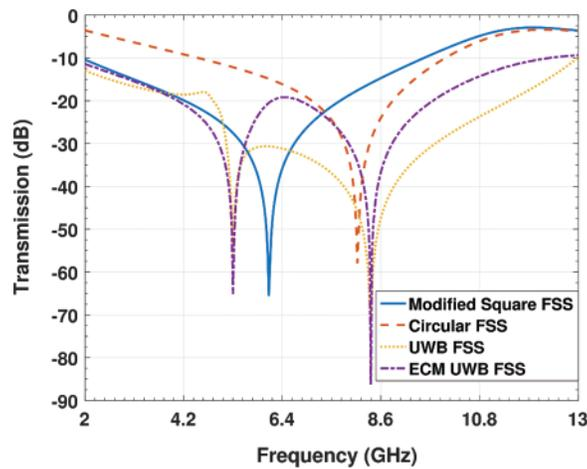
Figure 4: Simulation transmission results of MSLFSS, circular-loop, UWB FSS and ECM UWB FSS for 0° incidence
