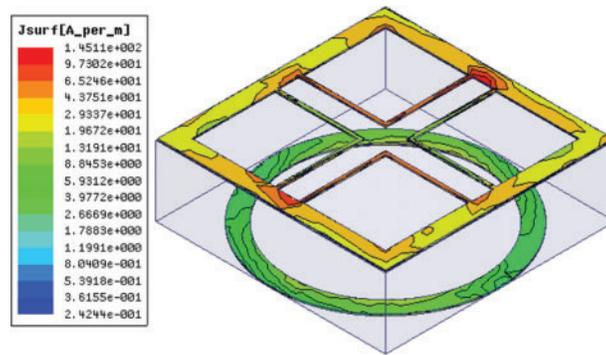
**Figure 6:** Distribution of electric current on the surface of square and circular element at center frequency 7.5 GHz
