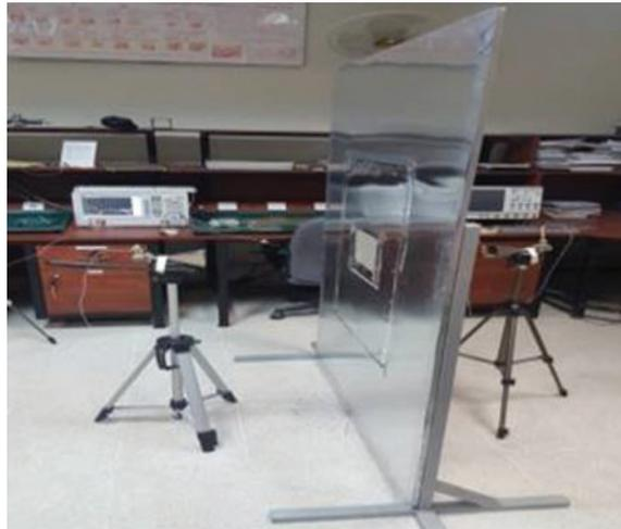
Figure 3: Experimental setup to measure the transmission response of the proposed FSS
