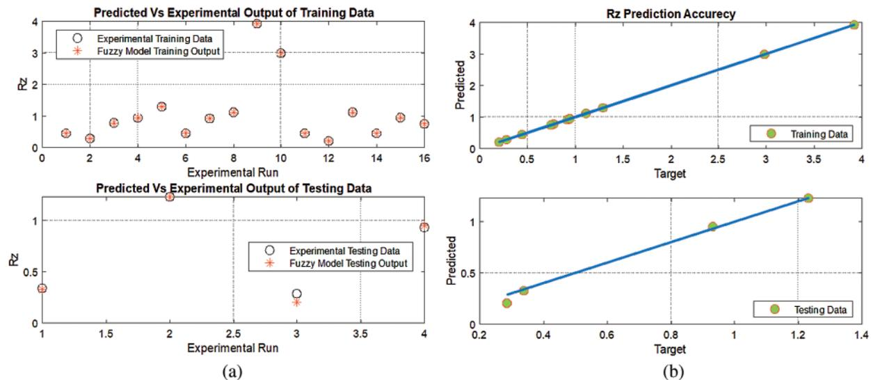
**Figure 7:** Comparison of the training and testing data: (a) predicted vs. experimental outputs of  $R_z$  and (b) prediction accuracy of training and testing data for  $R_z$
