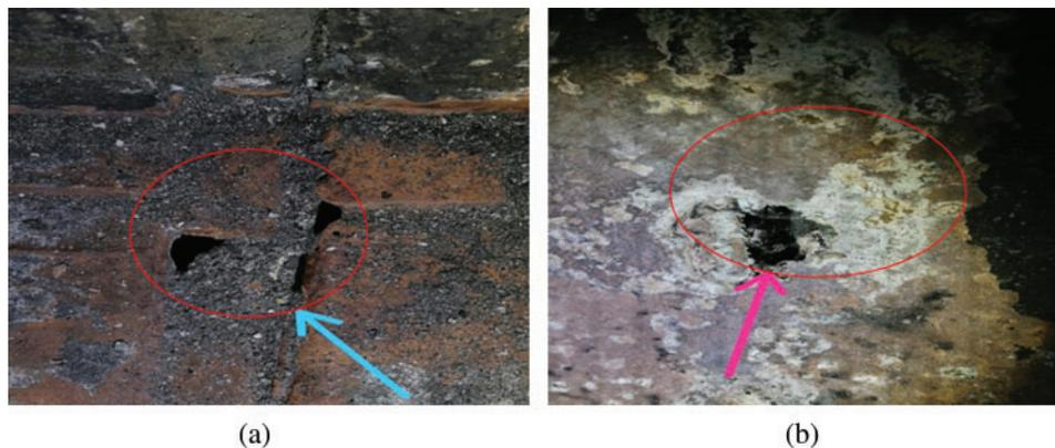
**Figure 1:** Mechanism for occurrence of corrosion in flue gas duct [1]. (a) Formation of cracks and holes inside flue duct (b) Formation of sulfuric acid
