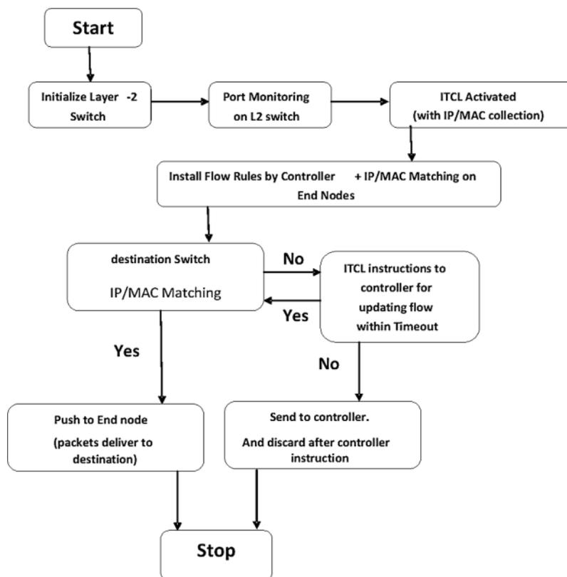
**Figure 3:** Data flow inside the implemented technique
