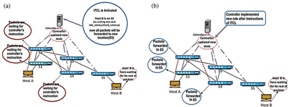
**Figure 2:** Packet forwarding techniques through destination host in proposed work (a) ITCL Layer instructing controller about movable host (b) all packets forwarded to changed location of destination host
