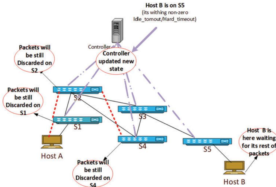
Figure 1: Packets discarded on all switches as per controller’s rule
