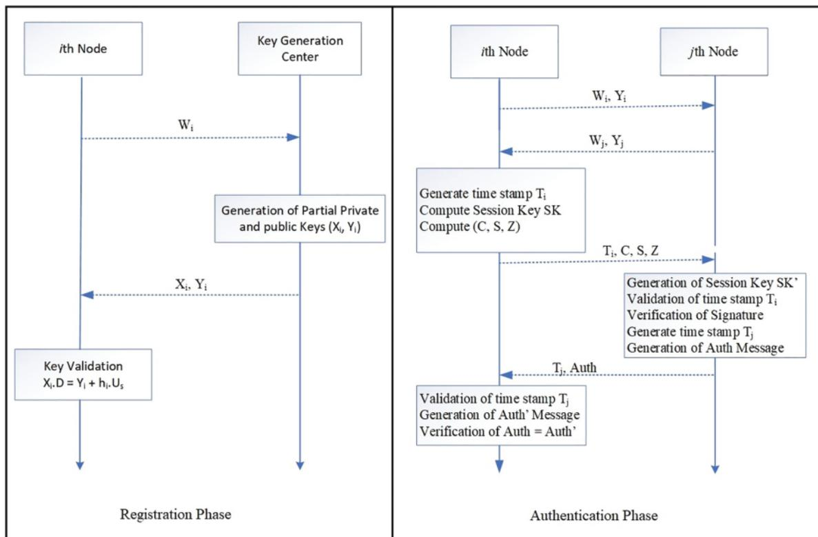
Figure 2: Flow of interaction in the proposed IIoT-CS scheme
