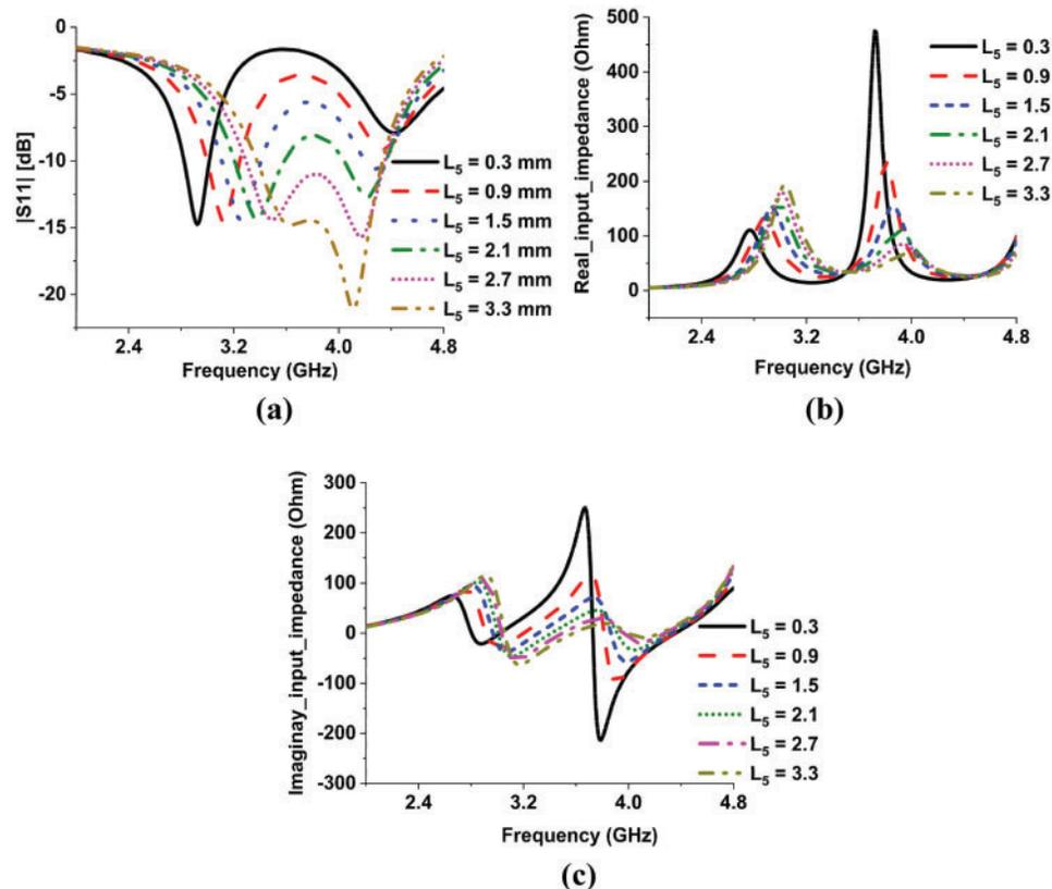
**Figure 12:** The parametric analysis of the split width on (a) reflection coefficient (b) real input impedance. (c) imaginary input
