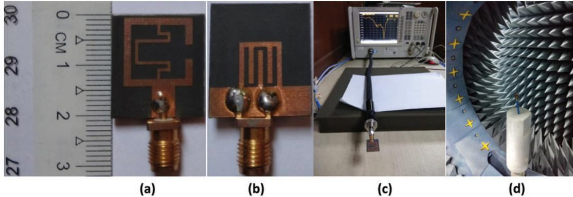
**Figure 13:** (a) Front side and (b) Back side of the antenna. (c) VNA measurement setup. (d) Satimo measurement setup
