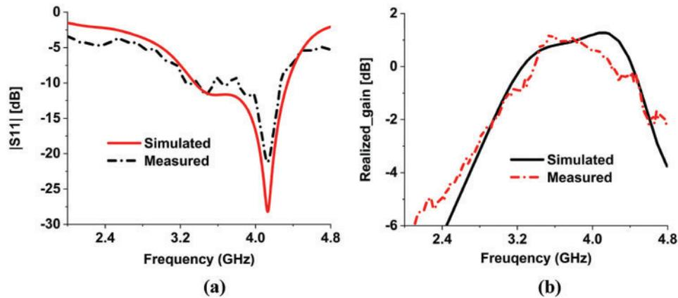
**Figure 14:** The simulated and measured (a) reflection coefficient and (b) realized gain of the proposed antenna
