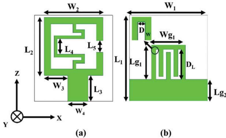
**Figure 1:** The configuration of the proposed antenna. (a) top view. (b) bottom view
