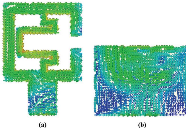
**Figure 9:** Current distribution without DGS (a) on the patch and (b) on the ground at 3.5 GHz
