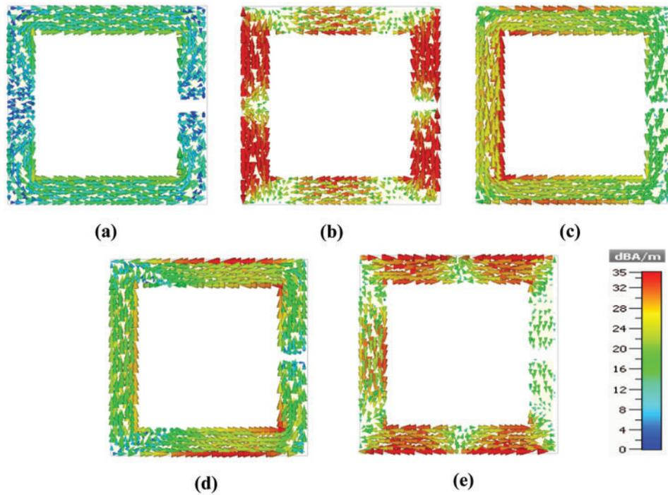
**Figure 4:** Current density at (a) 5.5 GHz for orientation 1. (b) 17 GHz for orientation 1. (c) 2.4 GHz for orientation 2. (d) 8.4 GHz for orientation 2. (e) 17 GHz for orientation 2
