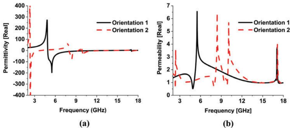
**Figure 2:** (a) Permittivity and (b) permeability of configuration (ii) for different orientations
