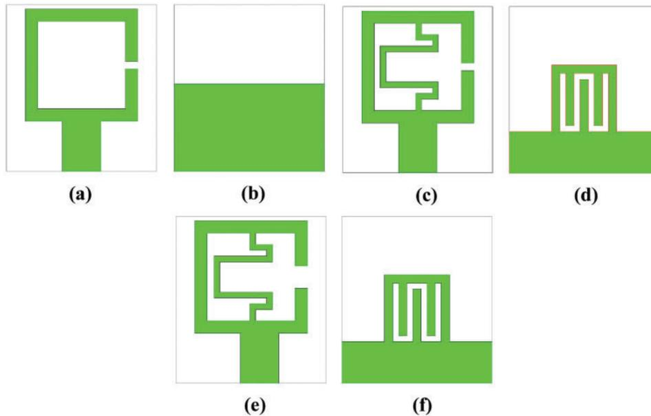
**Figure 7:** Design evolution of the proposed antenna. (a) patch of antenna 1. (b) ground of antenna 2. (c) patch of antenna 2. (d) ground of antenna 2. (e) patch of antenna 3. (f) ground of antenna 3
