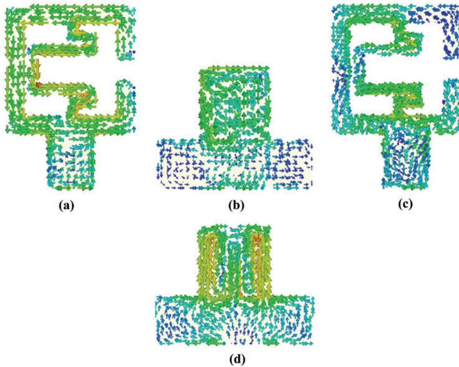
**Figure 10:** Current distribution with DGS (a) on the patch and (b) on the ground at 3.5 GHz. (c) on the patch and (d) on the ground at 4.13 GHz
