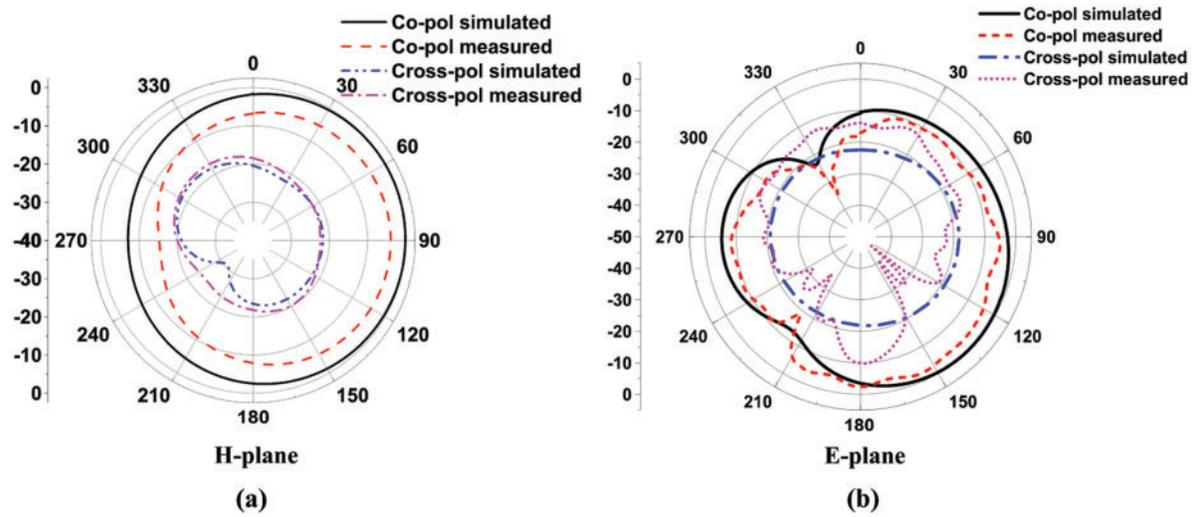
**Figure 15:** Simulated and measured radiation patterns of the proposed antenna. (a) XY-plane. (b) XZ-plane
