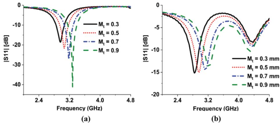
**Figure 8:** Parametric analysis of the meander line width (a) without DGS and (b) with DGS structure on reflection coefficient
