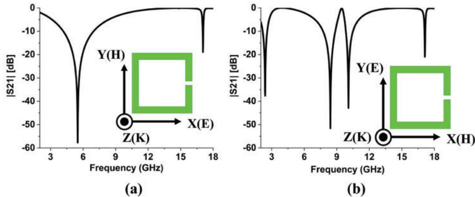
**Figure 3:** Transmission spectrum of the single-split resonator. (a) orientation 1. (b) orientation 2
