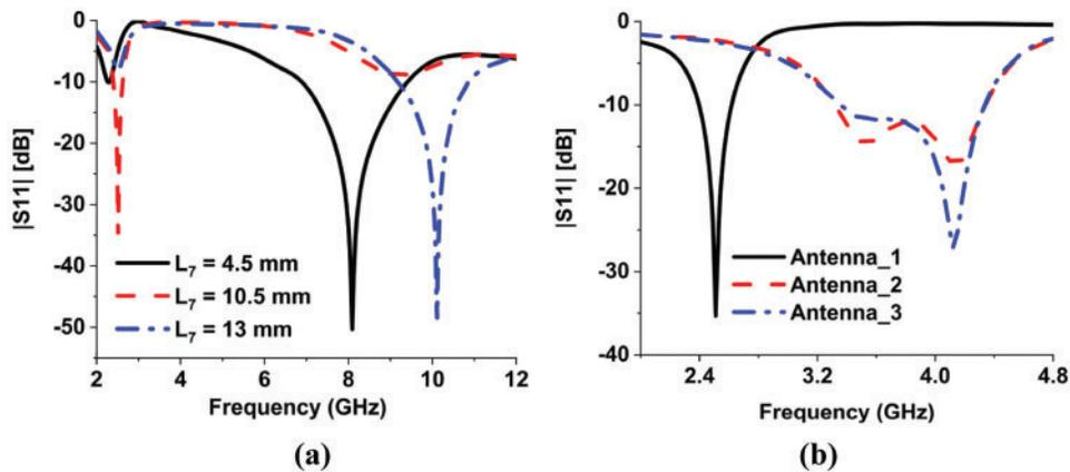
**Figure 6:** (a) Reflection coefficient of antenna 1 for different ground plane sizes. (b) comparison of reflection coefficient of 3 stages of the proposed antenna
