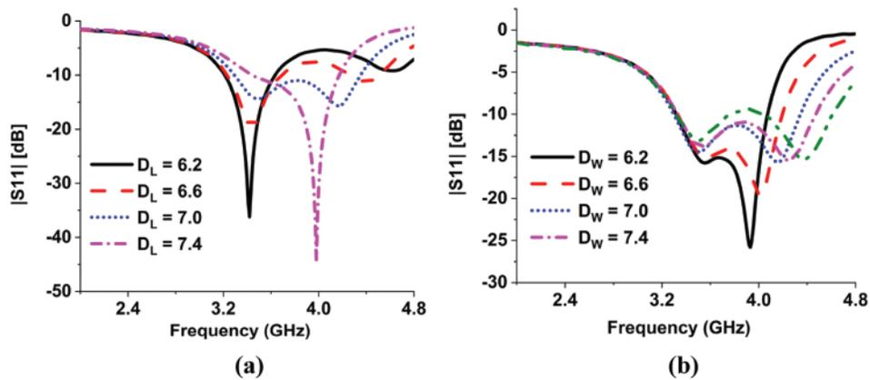
**Figure. 11:** Parametric analysis of the DGS (a) length and (b) width on reflection coefficient
