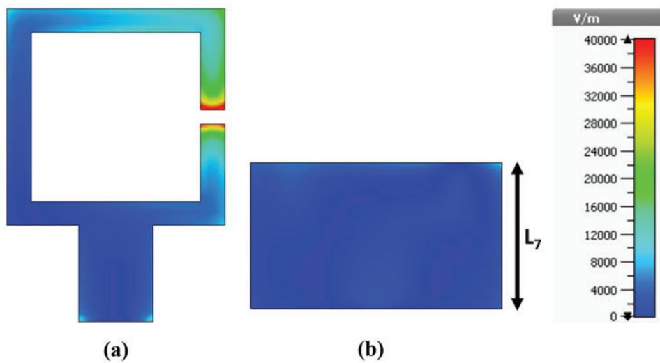
**Figure 5:** (a) Electric field distribution on the (a) patch and (b) ground of antenna 1 at 2.5 GHz
