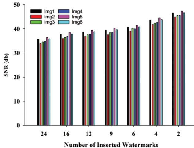
Figure 13: SNR comparison at different number of watermark insertion
