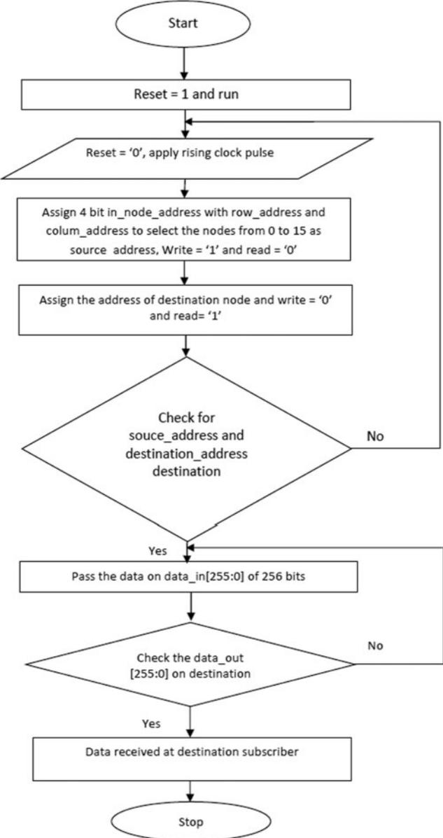
Figure 10: Flow chart for ring NoC
