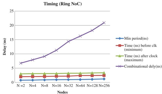
**Figure 12:** Timing values with cluster size in the ring NoC
