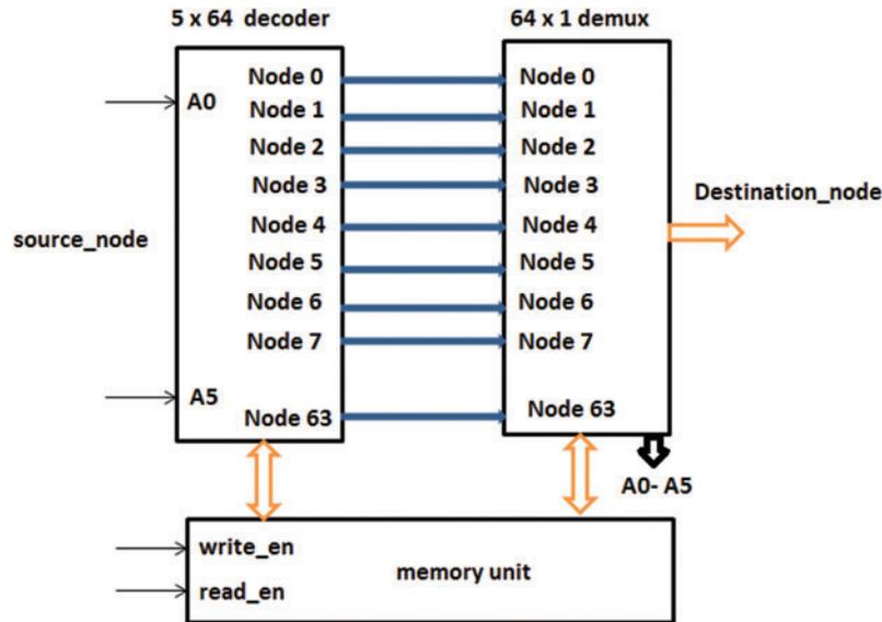
Figure 5: Datapath logic diagram [33]
