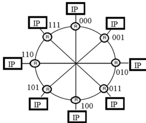
Figure 1: Ring NoC structure using 8 nodes
