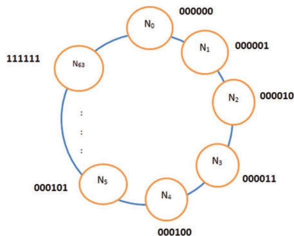
Figure 2: Ring NoC structure using 64 nodes [33]
