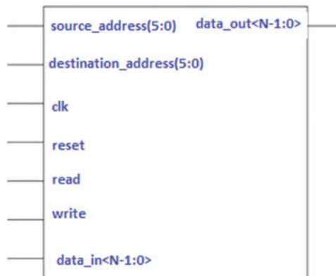
Figure 6: RTL view of ring NoC
