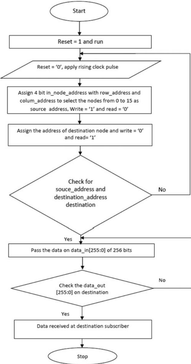
Figure 10: Flow chart for ring NoC
