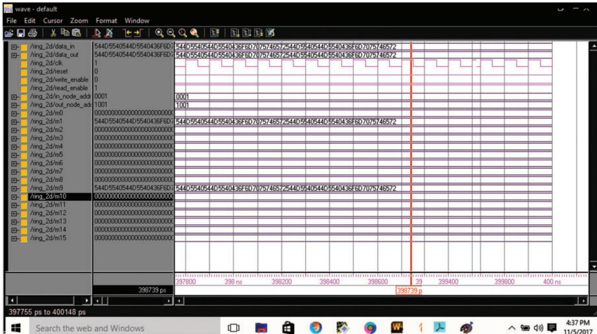
**Figure 8:** Modelsim result simulation of 256-bit data in hexadecimal for ring NoC
