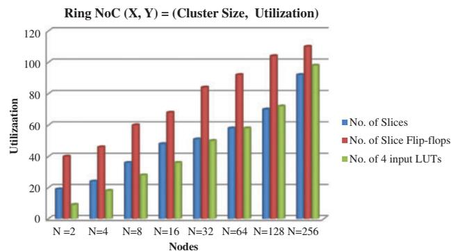
**Figure 11:** Hardware utilization with cluster size in the ring NoC
