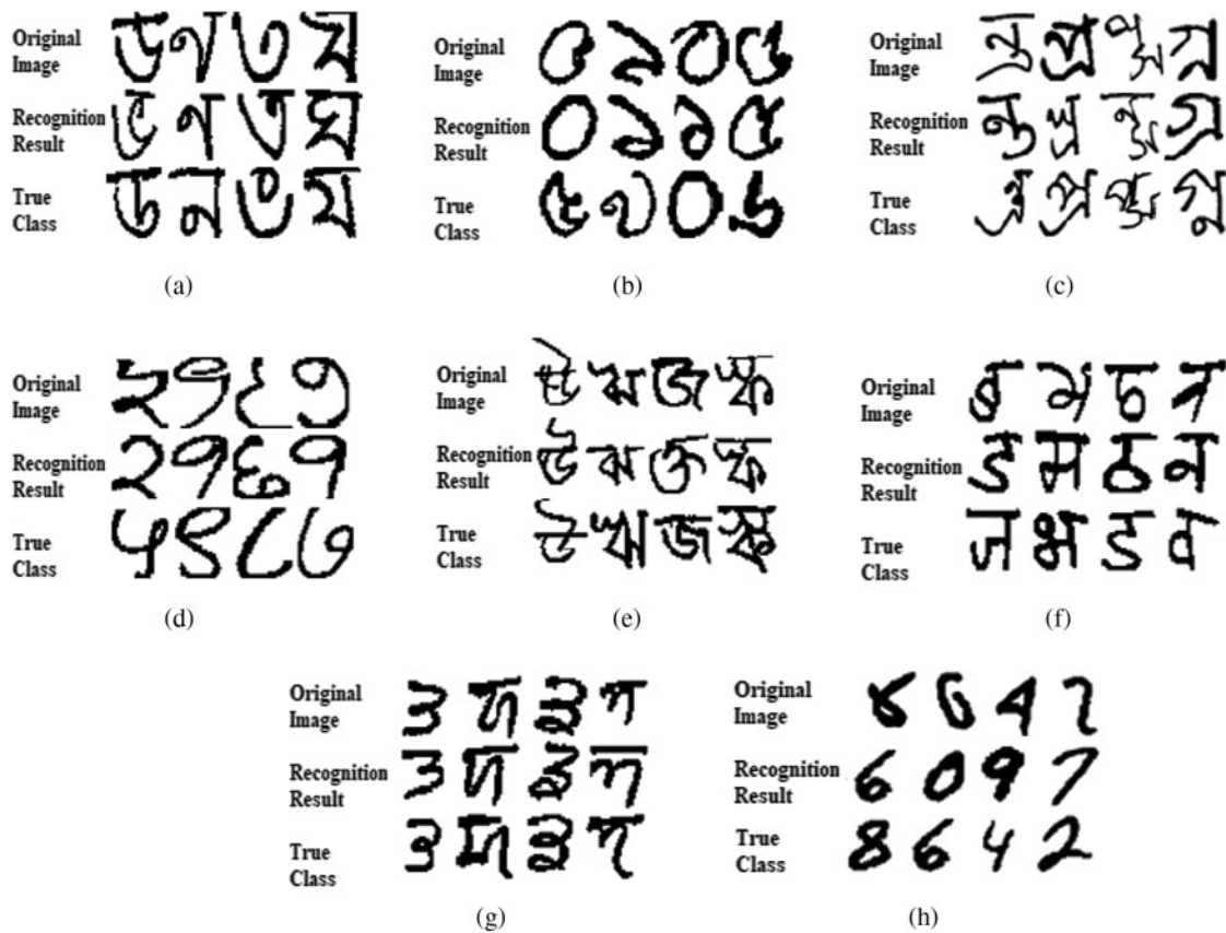
Figure 2: Illustration of frequently misclassified samples for the chosen benchmark datasets. (a) CMATERdb 3.1.1 (b) CMATERdb 3.1.2 (c) CMATERdb 3.1.3 (d) BanglaLekha-Iso (e) CMATERdb 3.2.1 (f) DHCD (g) DOGRA C-64 (h) MNIST
