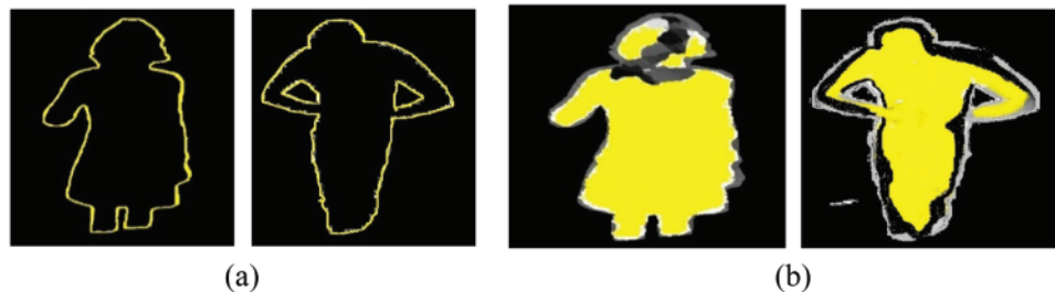
Figure 4: Ridge extraction of human silhouette (a) Binary edge extraction and (b) Ridge data generation
