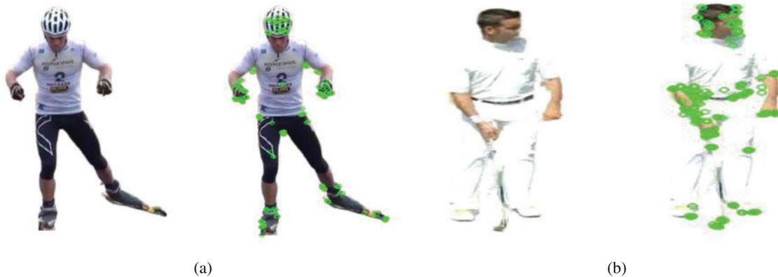
**Figure 5:** Results of applying an ORB feature descriptor. (a) skiing class–human silhouette (left) and its key feature points detected by ORB (right) and (b) golf class–human silhouette (left) and its key feature points detected by ORB (right)
