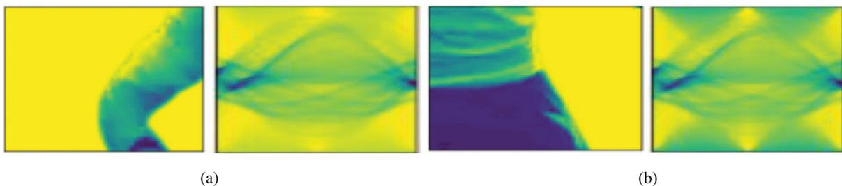
**Figure 6:** Radon transforms taken with respect to key points. (a) a window around the right elbow key point (left) and its radon transform (right) and (b) a window around the left hip key point (left) and its radon transform (right)
