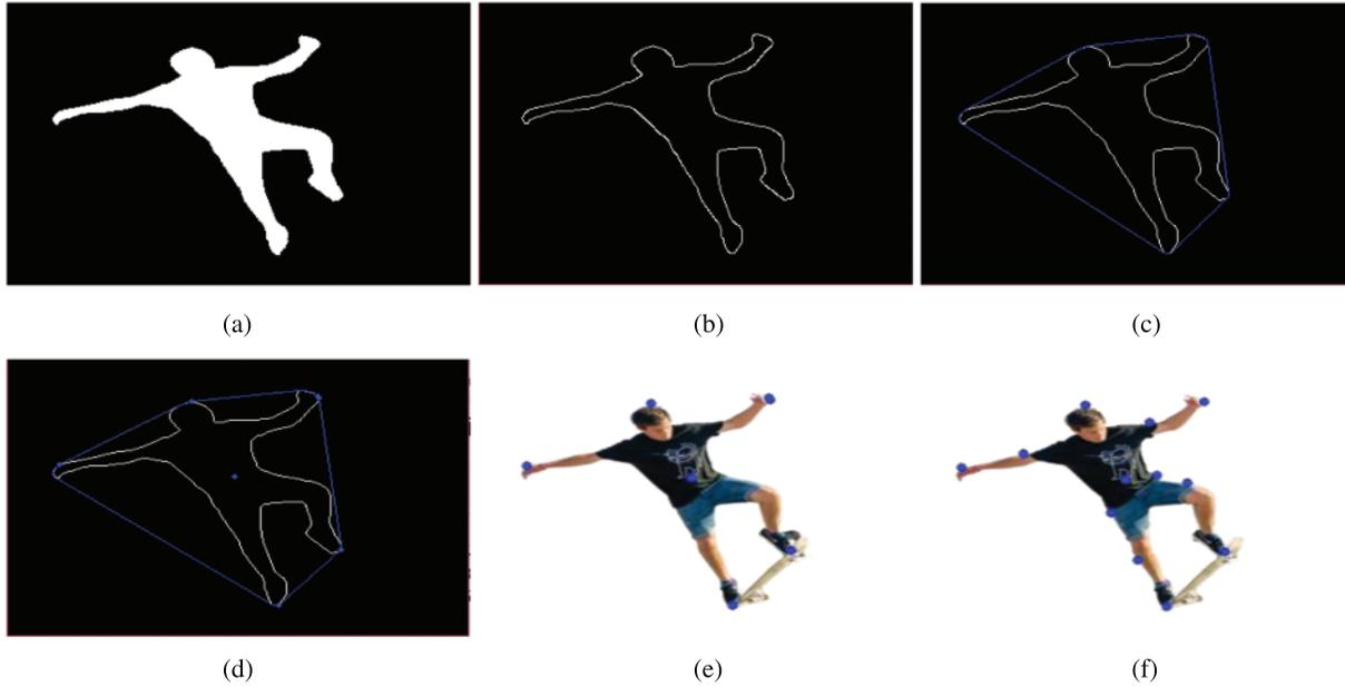
**Figure 4:** Results of key point detection. (a) segmented human silhouette, (b) silhouette contour, (c) convex hull around the silhouette, (d) convex hull vertices lying on the contour, (e) 6 detected key points, and (f) 12 extracted key points
