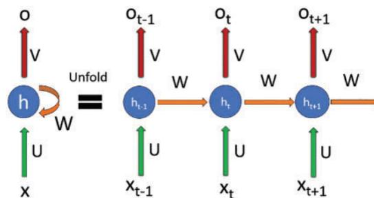
**Figure 2:** Illustration of forward propagation in recurrent neural network (RNN)
