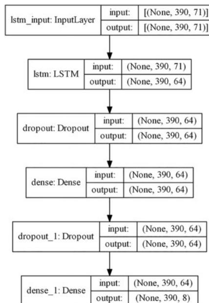
**Figure 4:** Model architecture of LSTM-RNN model
