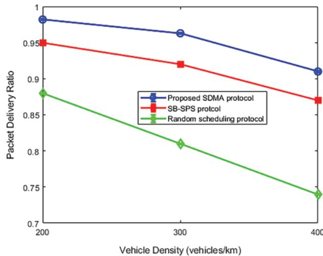
**Figure 3:** Packet delivery ratio at different vehicle densities
