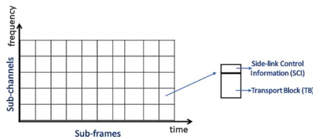
**Figure 1:** Frame and channel allocation in C-V2X
