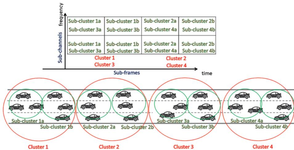
**Figure 2:** Proposed SDMA based C-V2X transmission
