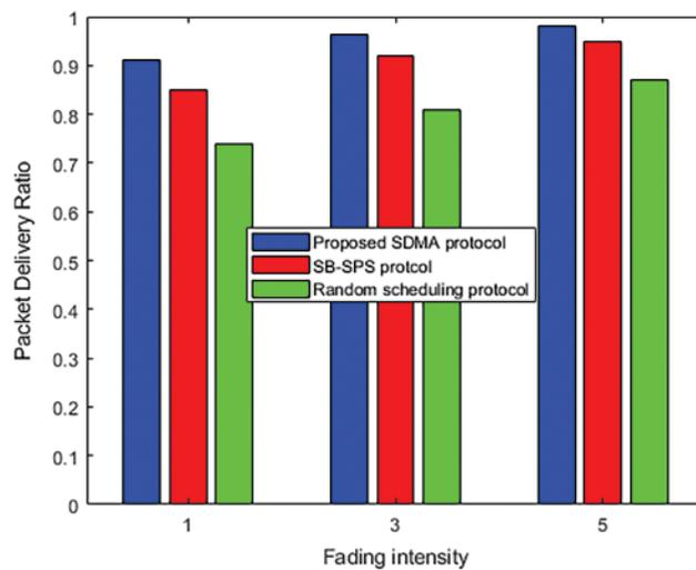
**Figure 5:** Packet delivery ratio at different fading intensities
