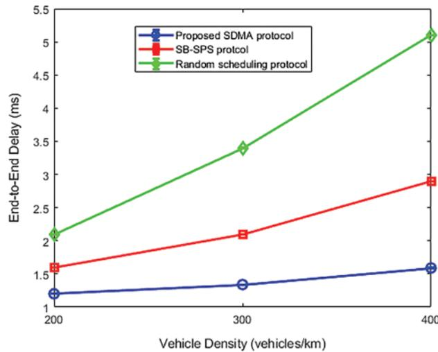
**Figure 4:** End-to-end delay at different vehicle densities
