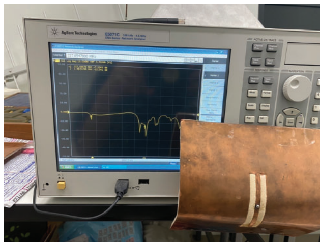
Figure 17: S_{11} of bending antenna without shorted circuit
