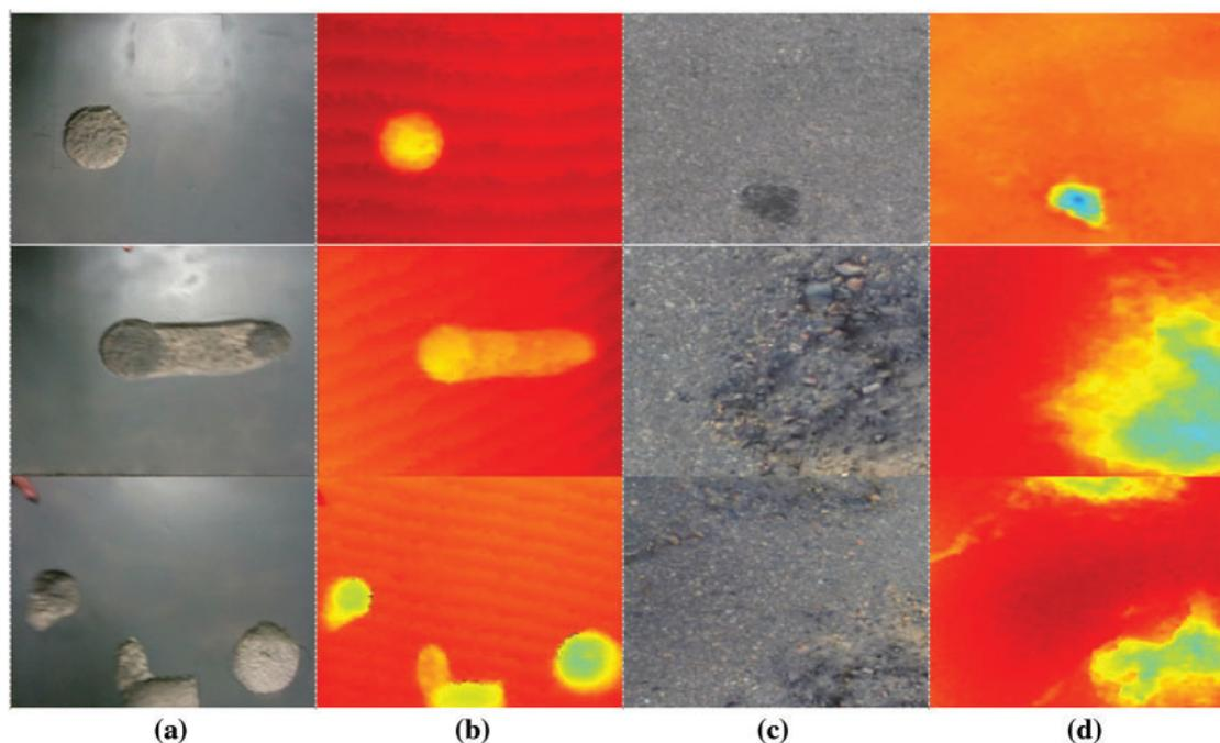
**Figure 3:** Examples of pothole synthetic data and Pothole 600 data: (a) RGB synthetic data, (b) TDM synthetic data, (c) RGB Pothole 600 data and (d) TDM Pothole 600 data
