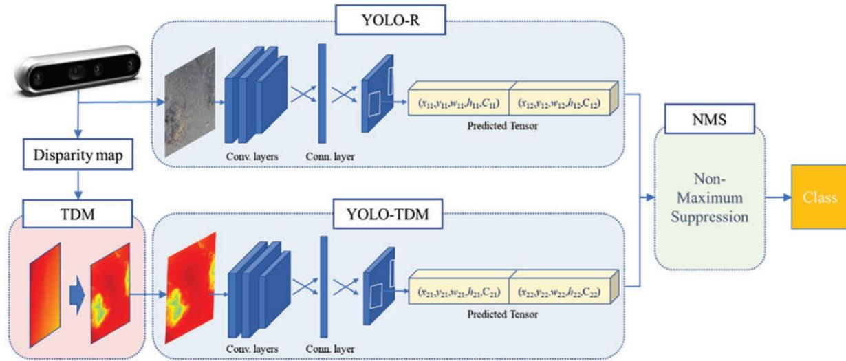
Figure 1: Block diagram of the proposed pothole detection system
