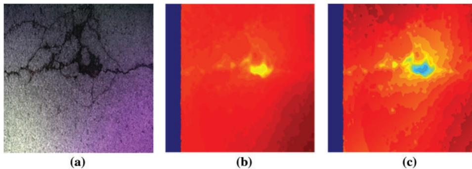
**Figure 2:** Example of a TDM conversion process: (a) raw image, (b) disparity map and (c) TDM
