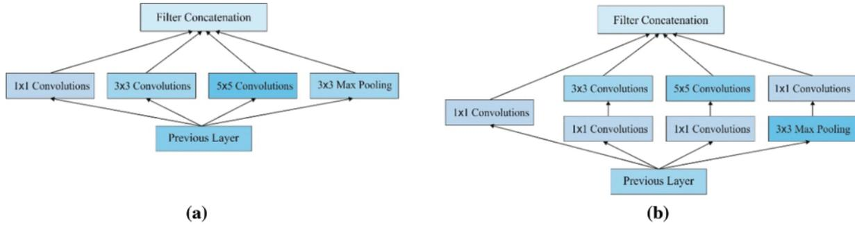
**Figure 3:** (a) Inception module naive version (b) Inception module with dimension reductions
