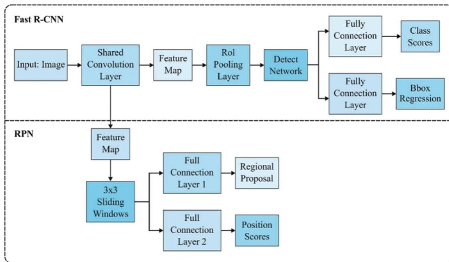
**Figure 2:** Process in Faster RCNN
