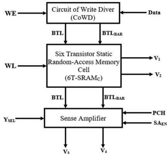
**Schematic 3:** Block diagram of cache memory design for single bit architecture
