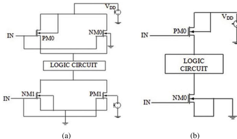
**Schematic 1:** (a) Low power reduction dual sleep technique circuit diagram, (b) Low power reduction sleep transistor technique circuit diagram
