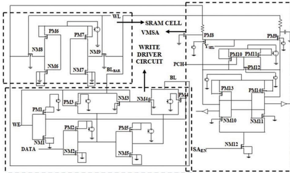
Schematic 6: Single bit 6T1SRAM<sub>C</sub> VDSA architecture circuit diagram
