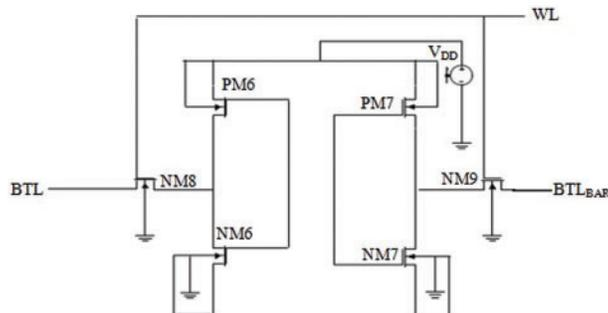
**Schematic 5:** 6TSRAM<sub>C</sub> circuit diagram
