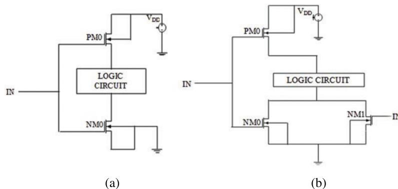
**Schematic 2:** (a) Low power reduction forced stack technique circuit diagram, (b) Low power reduction sleep stack technique circuit diagram
