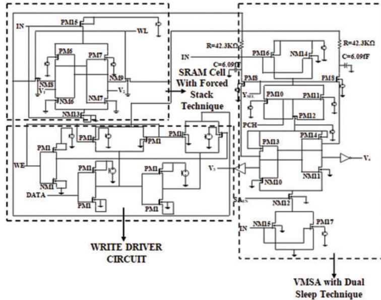
**Schematic 11:** Single bit 6T<sub>SRAM<sub>C</sub></sub> with LPRFST VDSA with LPRDST architecture circuit diagram
