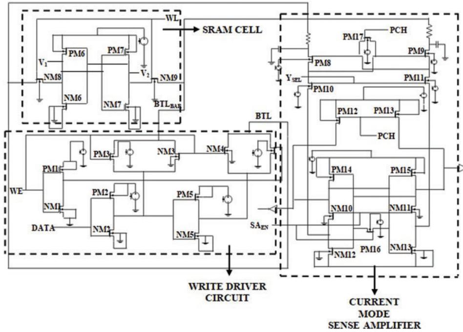
Schematic 7: Single bit 6T1SRAM<sub>c</sub> CDSA architecture circuit diagram
