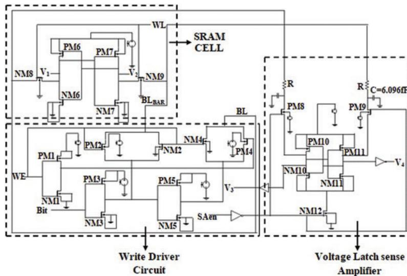
**Schematic 9:** Single bit 6T1SRAM<sub>C</sub> VLSA architecture circuit diagram
