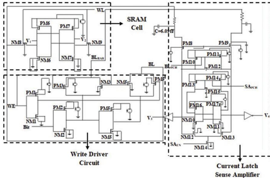
**Schematic 10:** Single bit 6T1SRAM<sub>c</sub> CLSA architecture circuit diagram
