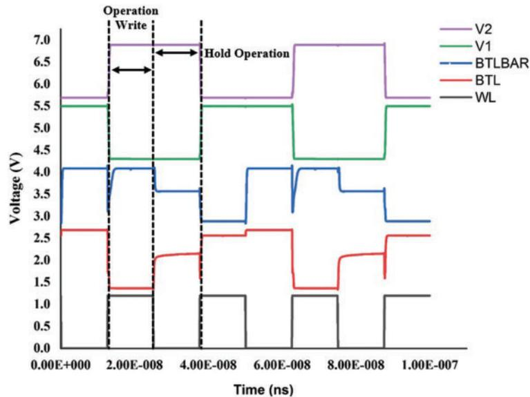
Schematic 13: 6TSRAM<sub>C</sub> output waveform
