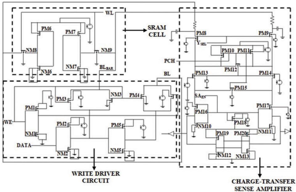
Schematic 8: Single bit 6T1SRAM<sub>c</sub> CTDSA architecture circuit diagram
