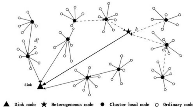
**Figure 4:** Deployment diagram of heterogeneous node in complex network
