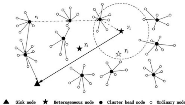
**Figure 7:** Heterogeneous node mobility diagram
