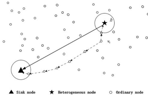
Figure 1: Network model with super link
