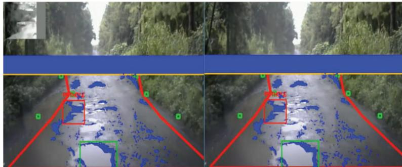
**Figure 4:** Road surface damage segmentation process
