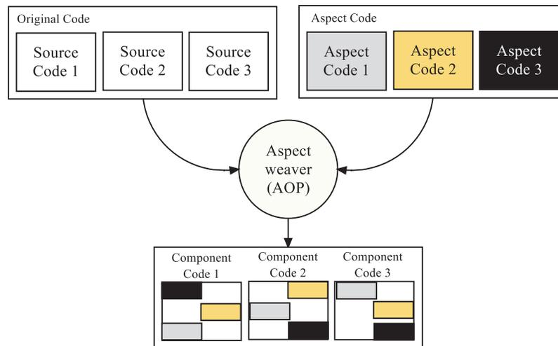
**Figure 1:** Weaving aspect module into original code
