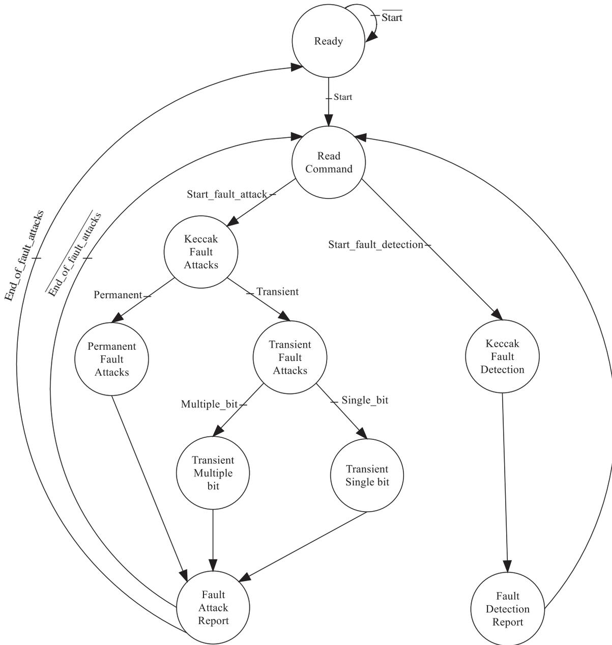
**Figure 3:** KFC finite state machine
