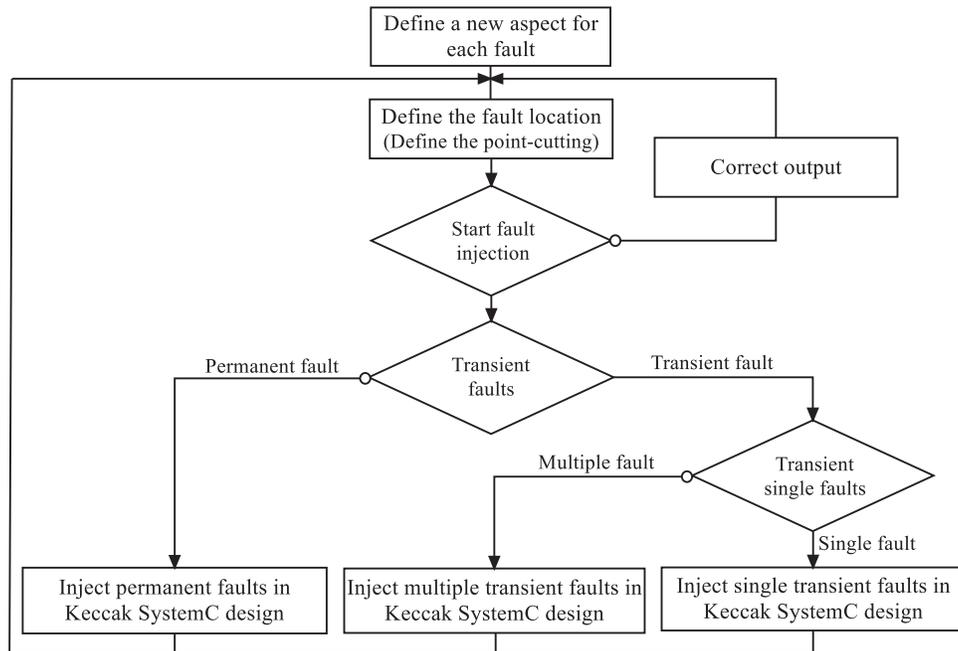
**Figure 4:** Aspect KECCAK fault injector flowchart
