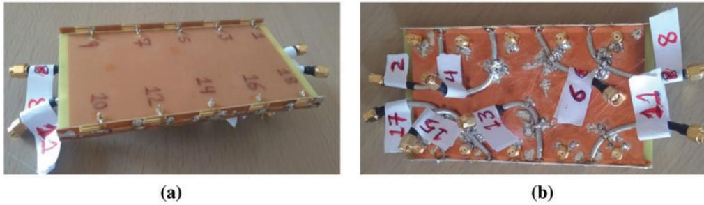
**Figure 7:** Fabricated Antenna prototype (a) Top view, (b) Bottom view
