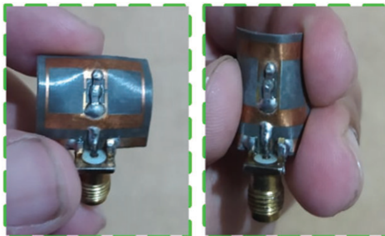
Figure 10: Antenna bending according to X and Y axis
