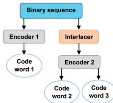
Figure 2: Parallel turbo encoder
