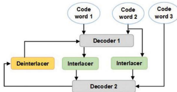
**Figure 3:** Parallel turbo decoder
