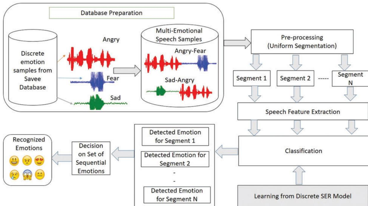
Figure 1: Proposed continuous SER work overflow
