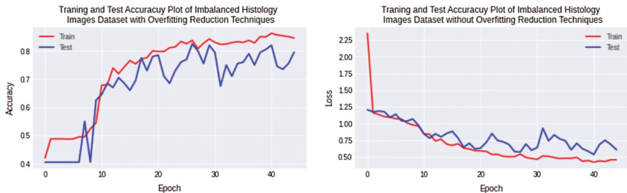
**Figure 8:** Training and testing accuracy plot on left side and loss error plot on the right side show overfitting reduction with a combination of imbalanced osteosarcoma image dataset with regularized CNN model
