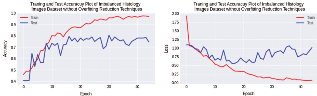
**Figure 6:** Training and testing accuracy plot on the left side and loss error plot on the right side show high overfitting for imbalanced Osteosarcoma images dataset by using non-regularized CNN model
