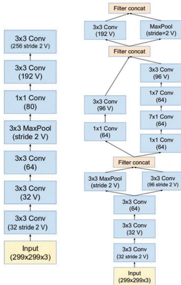
**Figure 5:** Architectures of InceptionResNet-V1(left), and InceptionResNet-V2 (right) [42]
