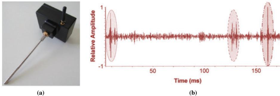
**Figure 3:** (a) TreeVibes device for recording palm tree sounds of pests [35], and (b) Graphical representation of three different impulses of detected RPW sounds
