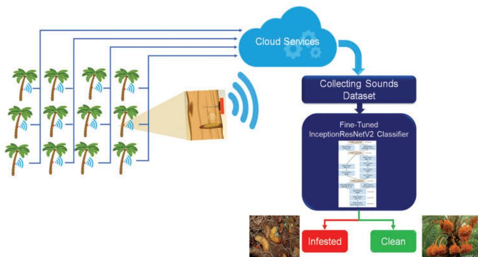
**Figure 6:** Schematic diagram of proposed IoT-based detection system of RPW sounds using fine-tuned InceptionResNet-V2 Classifier
