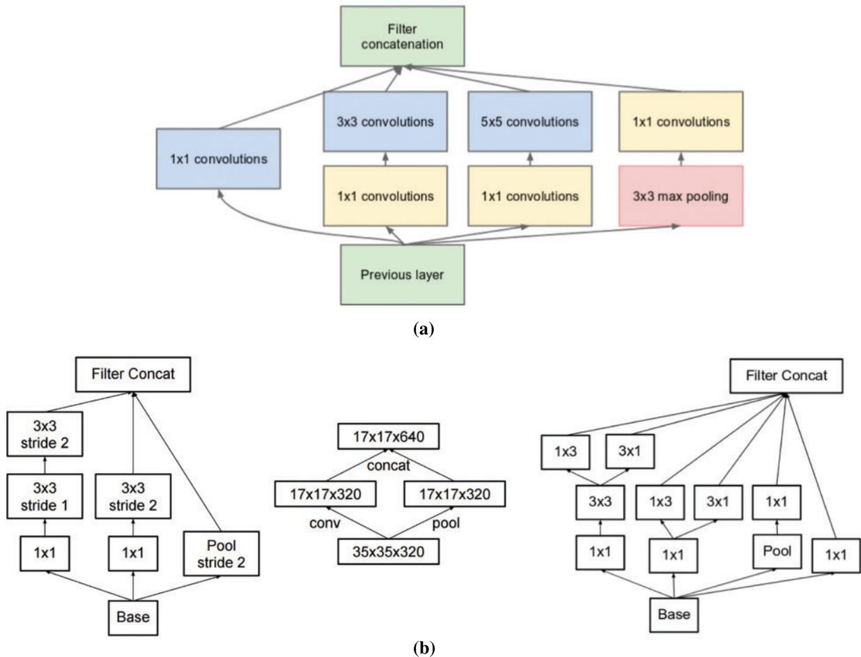
**Figure 4:** (a) Inception-V1 with dimensions reduction (GoogleNet) [40], and (b) Inception-V2 [41]
