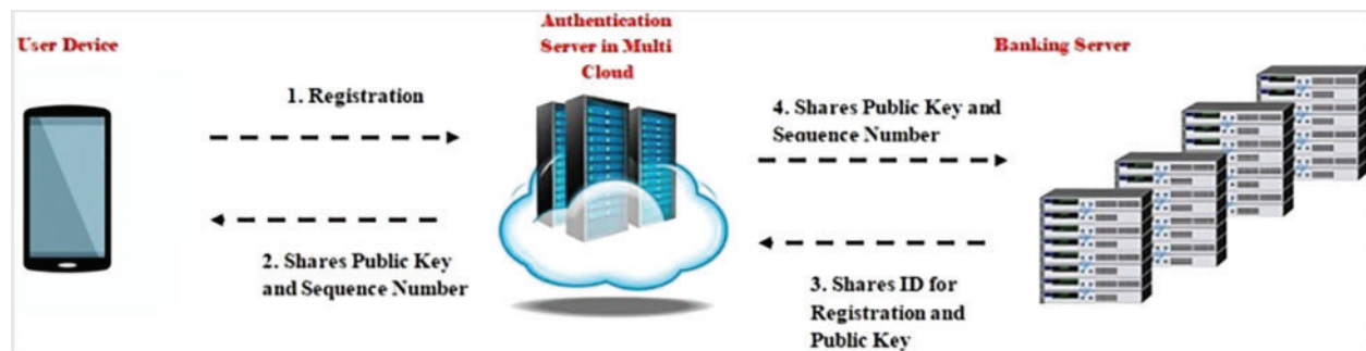
Figure 2: Message flow diagram- registration phase
