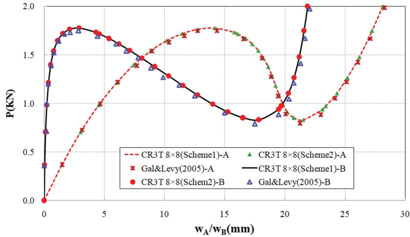
**Figure 8:** Load-displacement curves of the laminated cylindrical shell ( $0^\circ/90^\circ/0^\circ$ ) with  $t = 12.7$  mm
