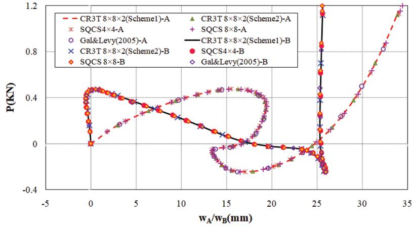
**Figure 6:** Load-displacement curves of the laminated cylindrical shell ( $0^\circ/90^\circ/0^\circ$ ) with  $t = 6.35$  mm
