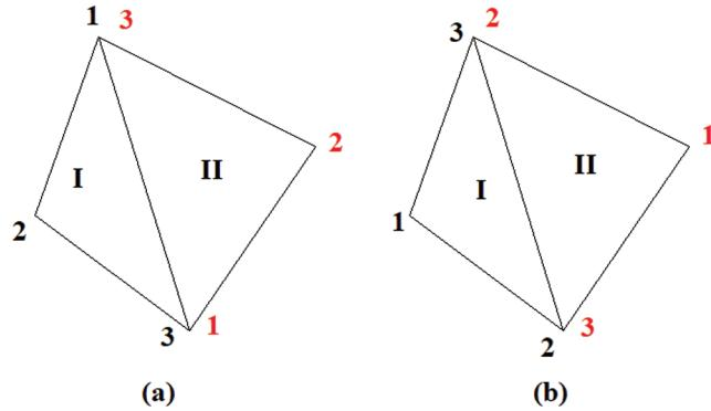
**Figure 2:** Two nodal numbering schemes, (a) Scheme 1; (b) Scheme 2
