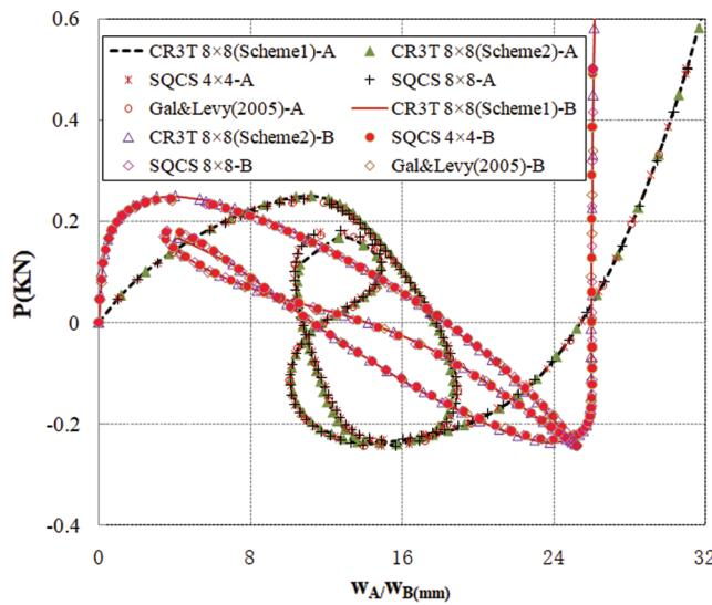
**Figure 5:** Load-displacement curves of the laminated cylindrical shell ( $90_4^0/0_4^0/90_4^0$ ) with  $t = 6.35 \text{ mm}$
