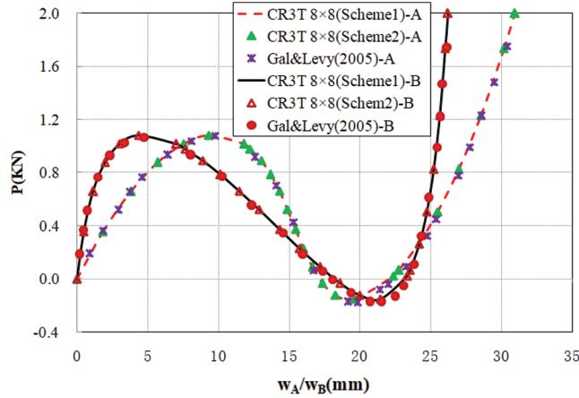
**Figure 7:** Load-displacement curves of the laminated cylindrical shell ( $90^\circ/0^\circ/90^\circ$ ) with  $t = 12.7$  mm
