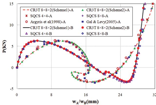
**Figure 11:** Load-displacement curves of the laminated cylindrical shell  $(45_2^\circ/-45_2^\circ)_6S$  with  $t = 6.35$  mm
