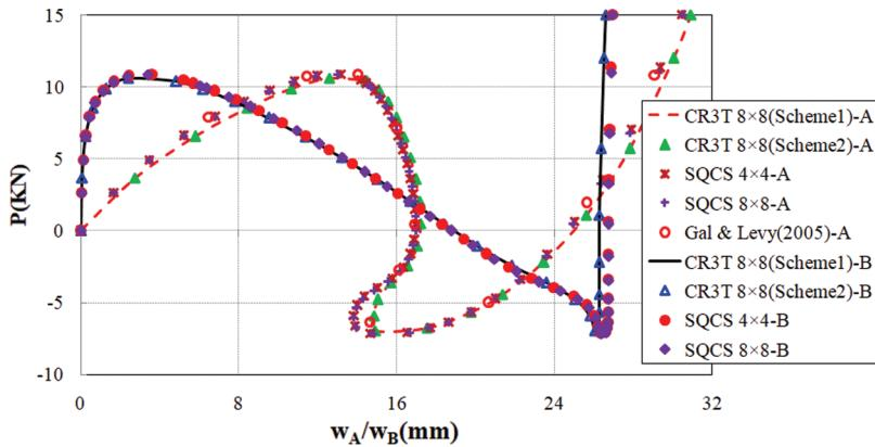
**Figure 10:** Load-displacement curves of the laminated cylindrical shell  $(45_2^\circ/-45_2^\circ/0_2^\circ/90_2^\circ)_3S$  with  $t = 6.35$  mm
