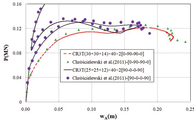
**Figure 17:** Load-displacement curves of the stiffened doubly curved cylindrical panel
