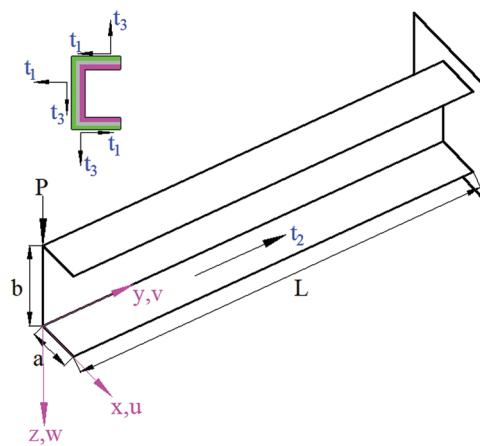
**Figure 12:** Geometry and loading of the three-layer channel section cantilever
