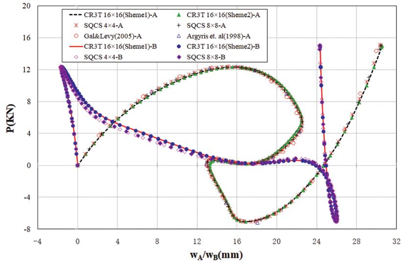
**Figure 9:** Load-displacement curves of the laminated cylindrical shell ( $0^\circ/90^\circ/0^\circ/90^\circ$ ) s with  $t = 6.35$  mm
