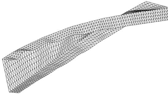
**Figure 14:** Deformed shape of the laminated channel section cantilever (0°/90°/0°)
