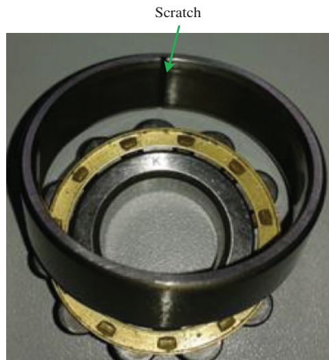
Figure 4: Bearing outer ring fault
