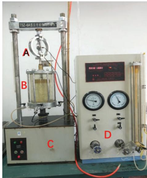
**Figure 4:** TSZ-6A triaxial apparatus A: force gauge; B: pressure cell; C: axial loading system; D: confining pressure control system
