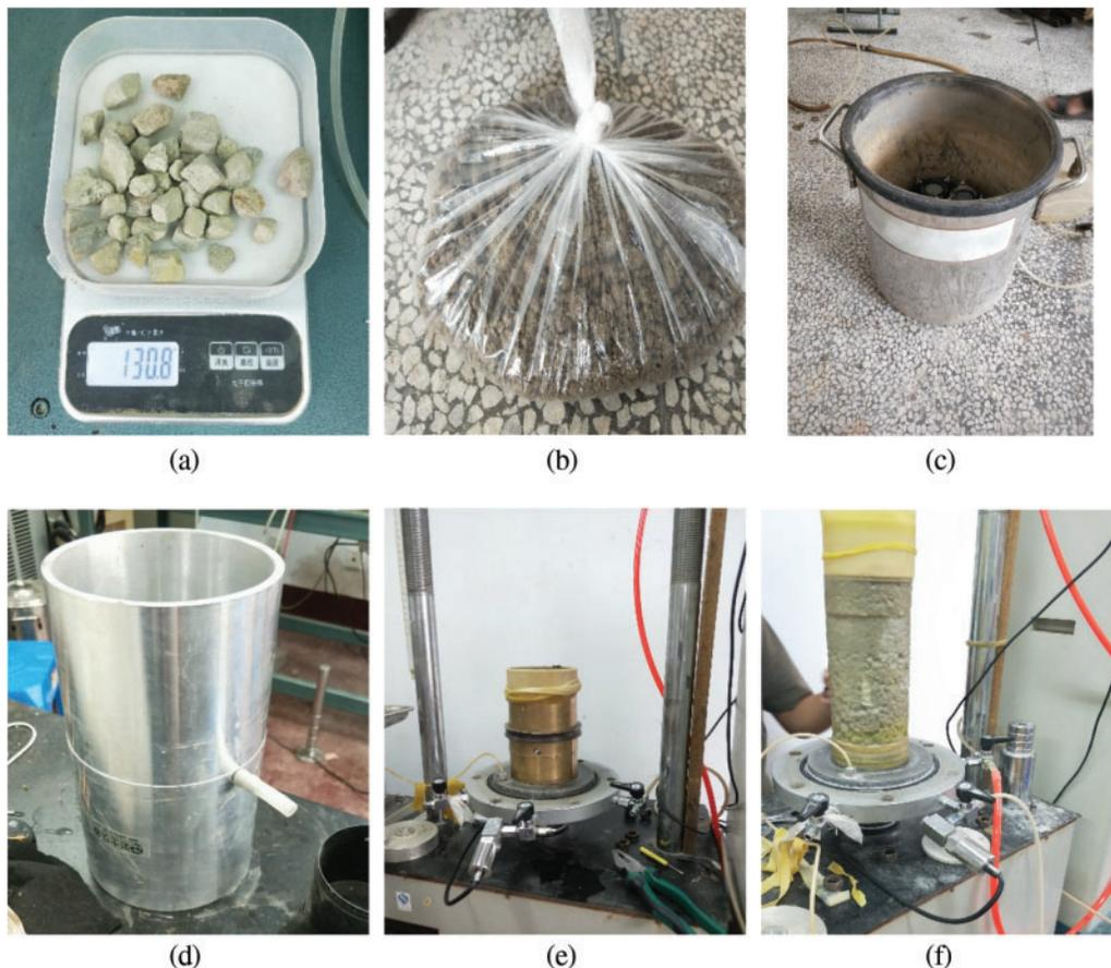
**Figure 3:** Processes of specimen preparation (a) weigh according to the proportion; (b) sealed and stored; (c) vacuum saturation; (d) bearing membrane tube; (e) compacted in three layers; (f) saturated with air extractor
