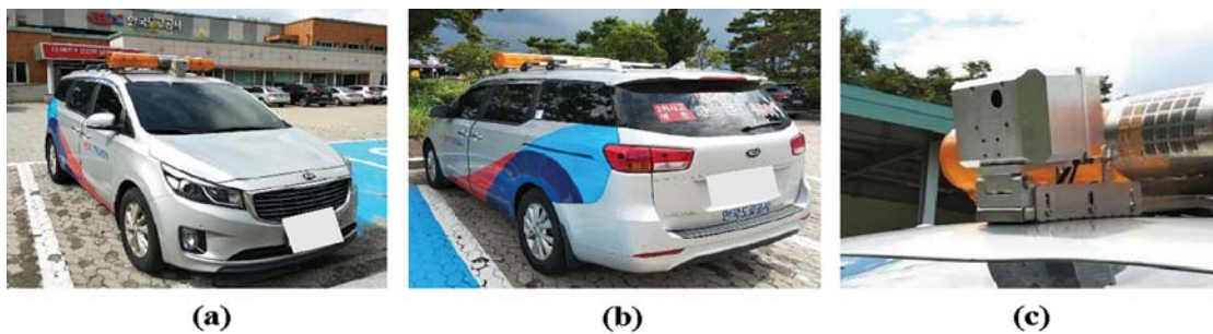
Figure 9: PotholeEye + installed on a vehicle to check the road surface; (a) front view; (b) back view; (c) cover for a camera exposed to the outside
