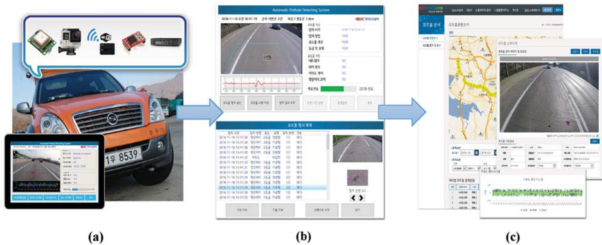
Figure 1: Conceptual diagram for real-time road pavement distress detection; (a) data collection step, (b) real-time detection step, and (c) detected image recording step
