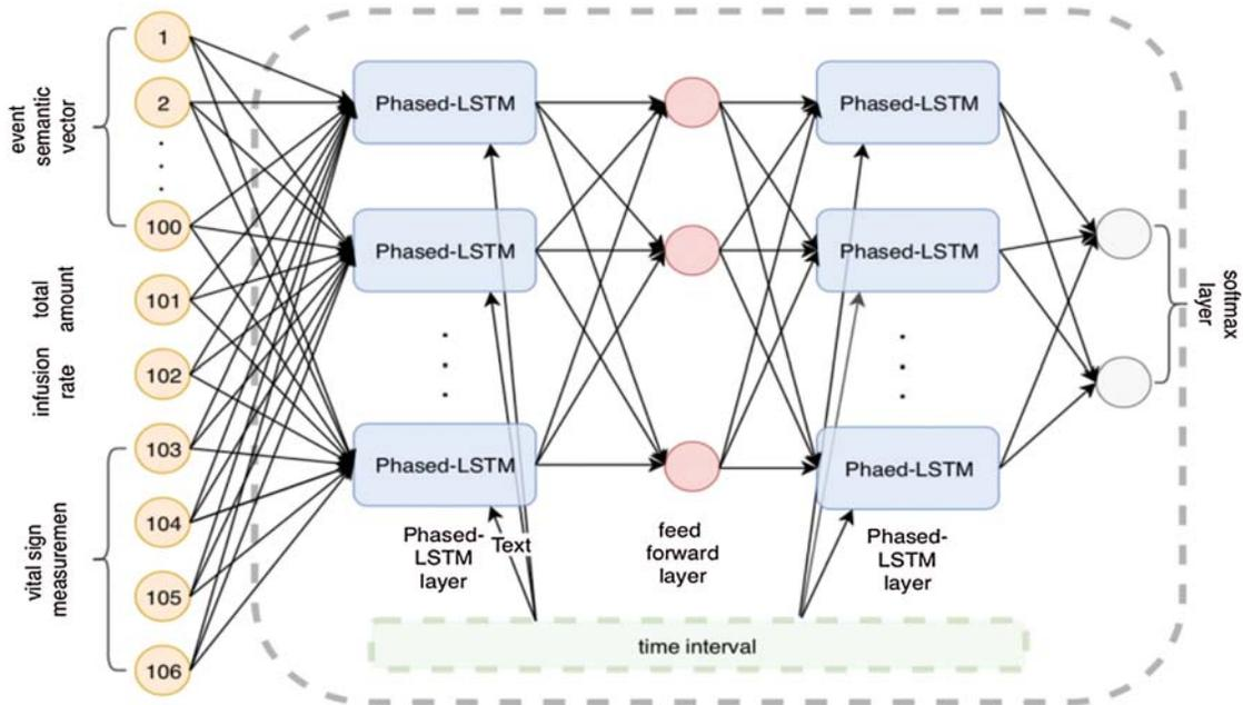
**Figure 8:** The architecture design of Phased-LSTM based model
