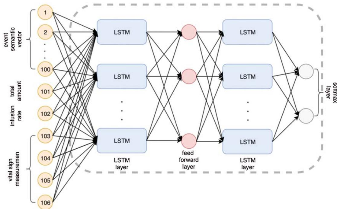
**Figure 7:** The architecture design of LSTM based model
