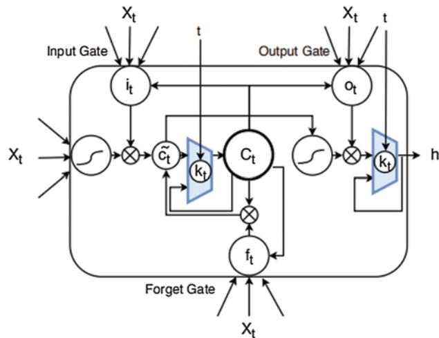
**Figure 6:** The architecture of Phased-LSTM cell
