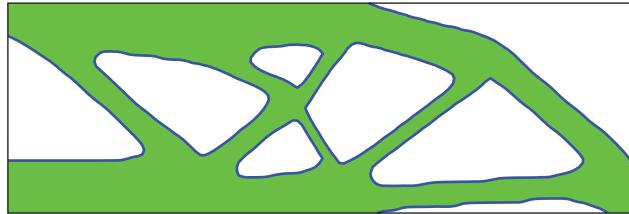
**Figure 9:** The optimized structure with the Lagrange multiplier being determined by using the augmented Lagrange multiplier method. Compliance of the optimized structure is 187.36, and volume is 3.00
