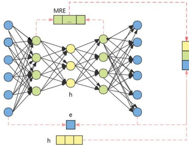
**Figure 3:** The procedure of MRE, where green points denote hidden layer neuros, yellow points are compressed features, and blue points are input and output data point
