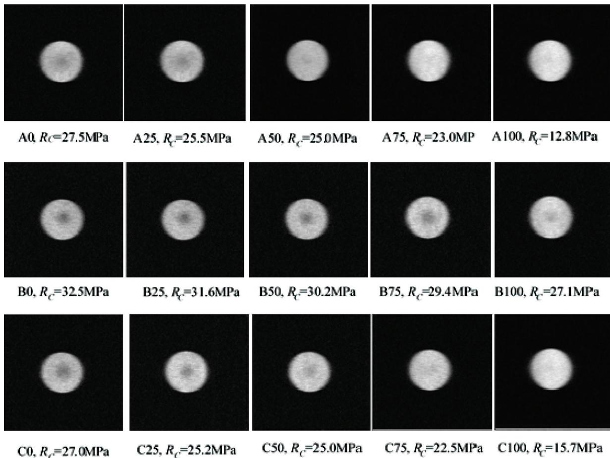
**Figure 2:** Relationship between the NMR images of different rock samples and their uniaxial compressive strength values
