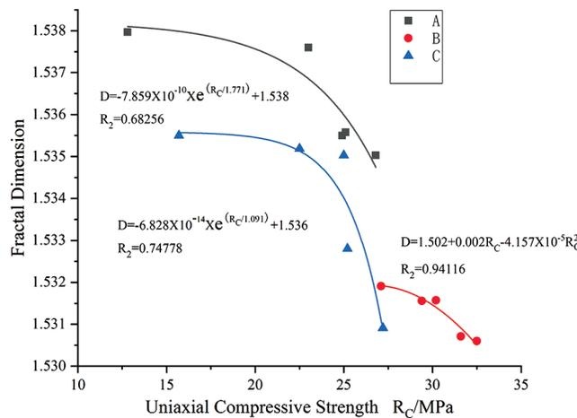
**Figure 4:** Relationship between the fractal dimension and uniaxial compressive strength of white sandstone under coupling effects
