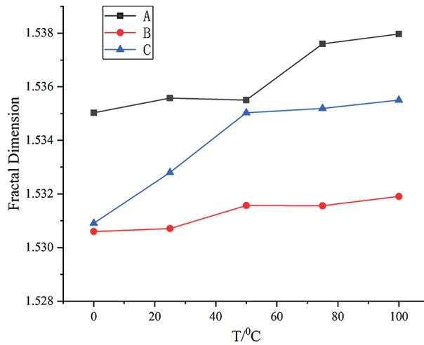
**Figure 3:** Variation of the fractal dimension (D) under different coupling effects of chemical corrosion and temperature
