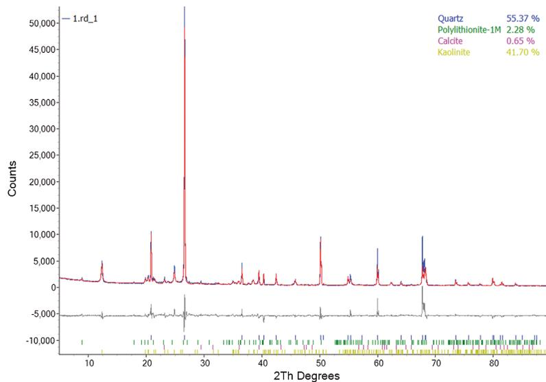
**Figure 1:** XRD spectra of the white sandstone samples
