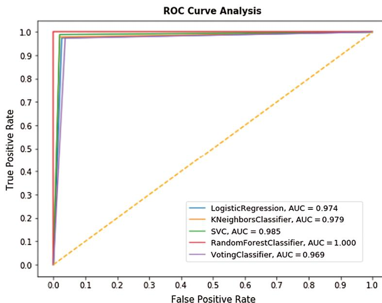
**Figure 8:** ROC analysis of ensemble model with different ML methods
