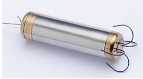
Figure 5: Miniaturized endocardial electromagnetic energy harvester
