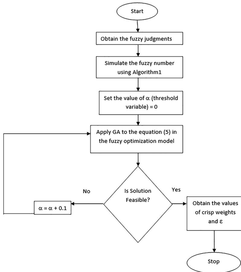
Figure 4: Working of the proposed technique
