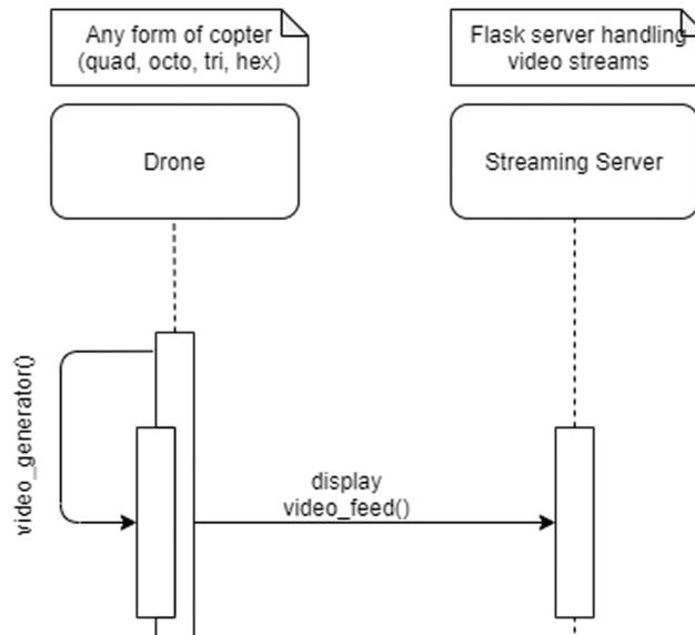
**Figure 10:** Drone broadcasting camera feed sequence diagram
