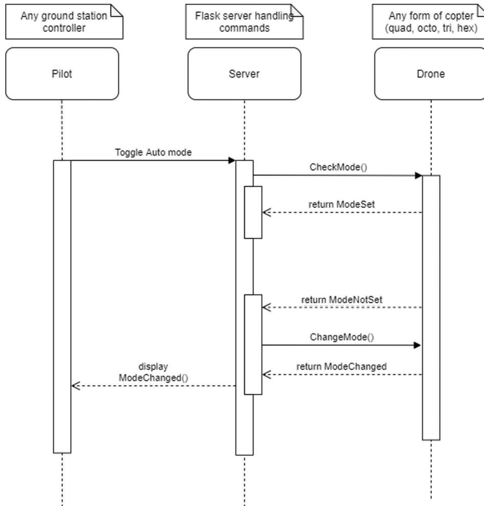
**Figure 8:** Mode change sequence diagram
