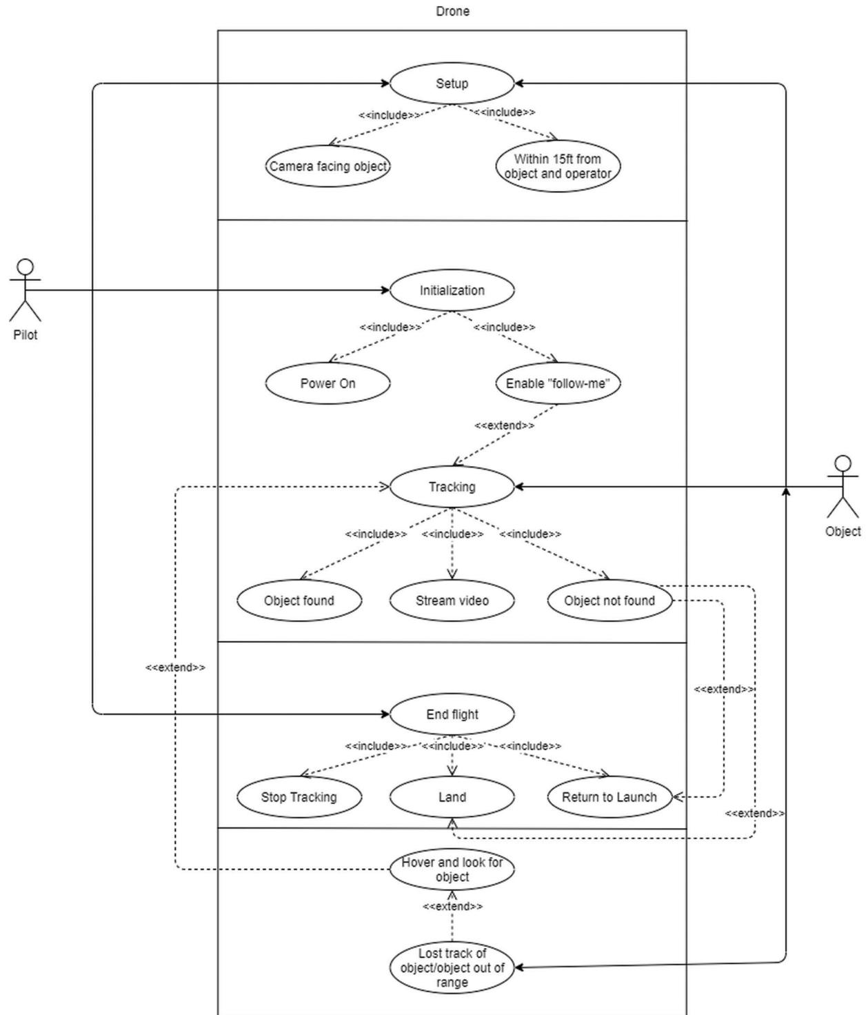
**Figure 6:** Interaction between the drone, the pilot and the tracked object
