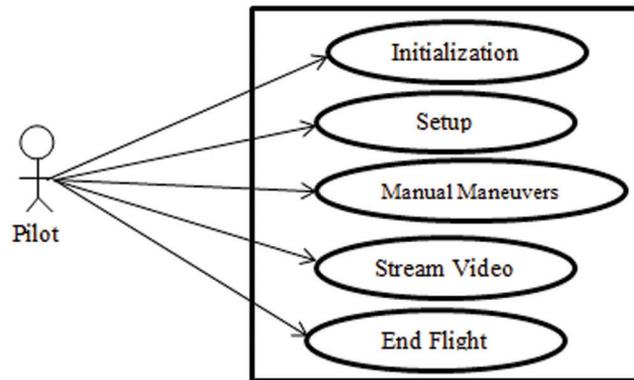
**Figure 3:** Pilot’s use case diagram
