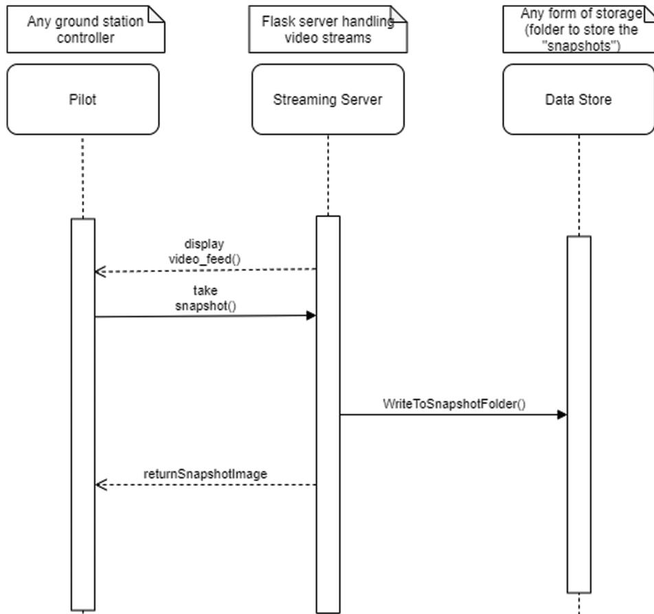
**Figure 9:** Pilot streaming live drone broadcast sequence diagram
