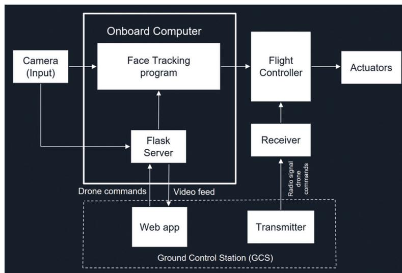
**Figure 1:** Block diagram showing the logical design of the proposed system
