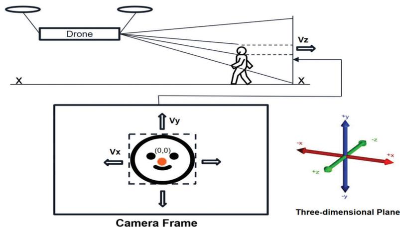
**Figure 2:** Face tracking procedure schematics
