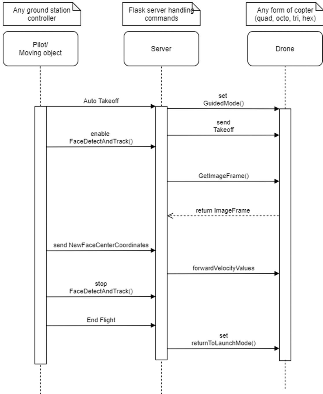
**Figure 7:** Object tracking sequence diagram
