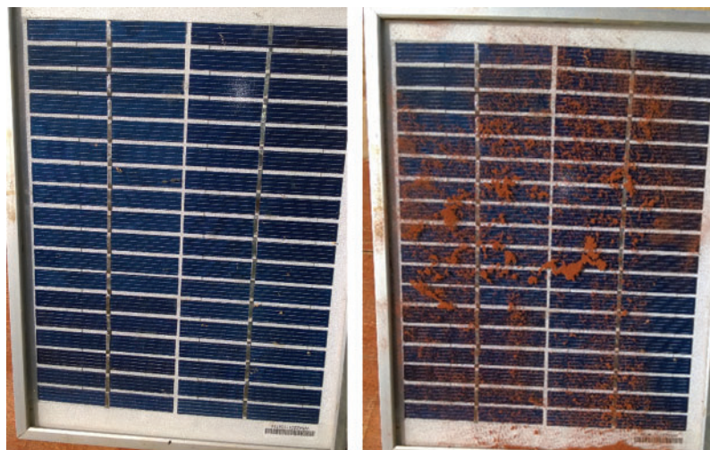
(a) Solar PV panel without dust
