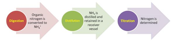
Figure 2: Kjeldahl step-wise process into three steps: Digestion, neutralization, and titration
