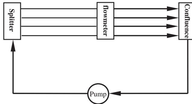
**Figure 1:** Original splitter experimental system diagram
