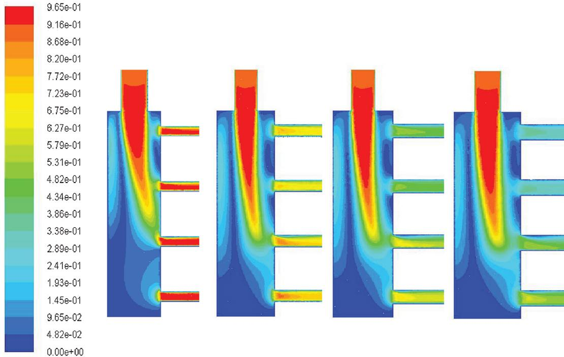
**Figure 6:** Velocity comparison cloud diagram corresponding to the inner diameters of different outlets when the inner diameter of the shunt chamber was 25 mm
