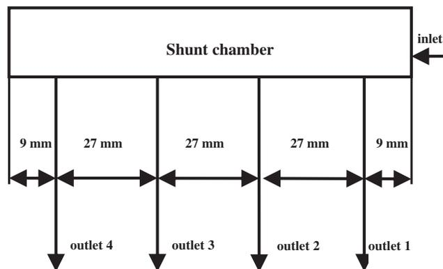
**Figure 2:** Schematic diagram of the center distance structure of the original splitter outlet
