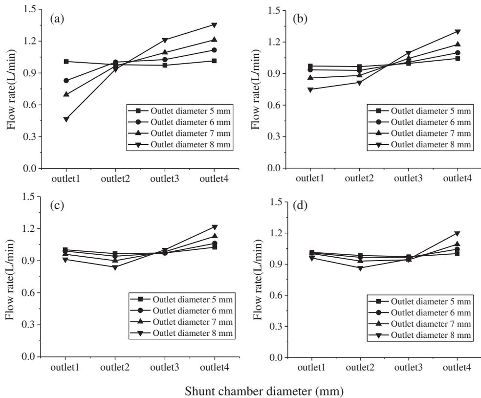
**Figure 8:** Dependence of the flow rate of each outlet on the inner diameter of the shunt chamber and outlet (a) 20 mm (b) 25 mm (c) 30 mm (d) 35 mm
