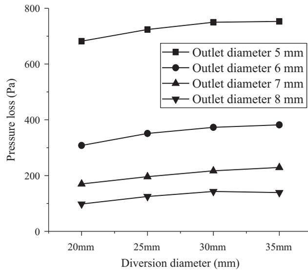
**Figure 10:** Pressure loss graphs for different models
