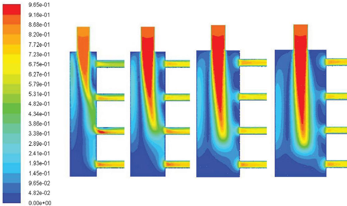
**Figure 7:** Velocity comparison cloud diagram corresponding to the inner diameter of different shunt chamber when the inner diameter of the outlet is 6 mm
