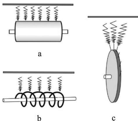
**Figure 1:** Rotary needleless electrospinning equipment. (a) A rotary cylinder spinneret [18], (b) A spiral coils spinneret [19], (c) A Needle-disk electrospinning setup [12]
