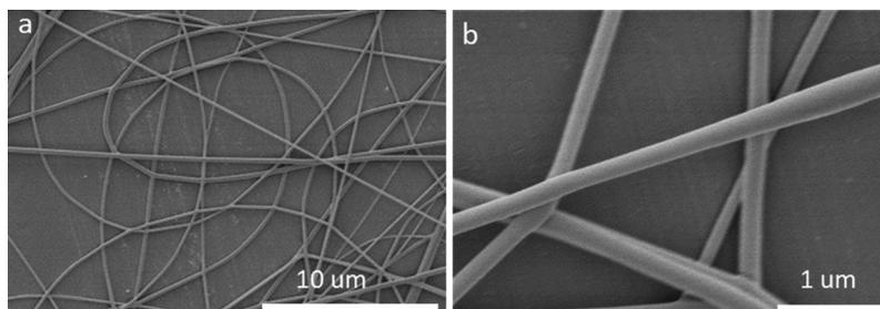
**Figure 3:** SEM images of PVA nanofibers. (a) SEM image at low multiple. (b) SEM image at high multiple
