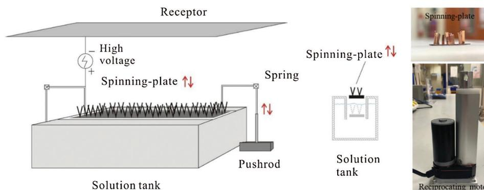
**Figure 2:** Reciprocating needleless electrospinning setup
