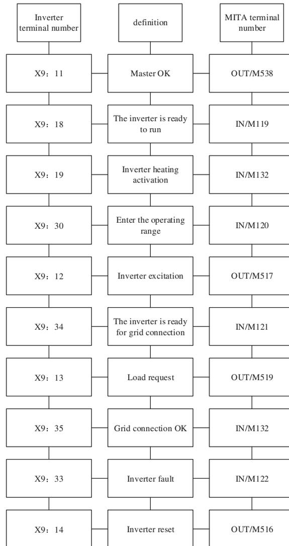
**Figure 2:** Communication control information between variable-frequency drive and main controller of wind turbine
