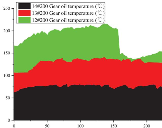
**Figure 4:** Temperature comparison curve of three groups of prototype gearboxes
