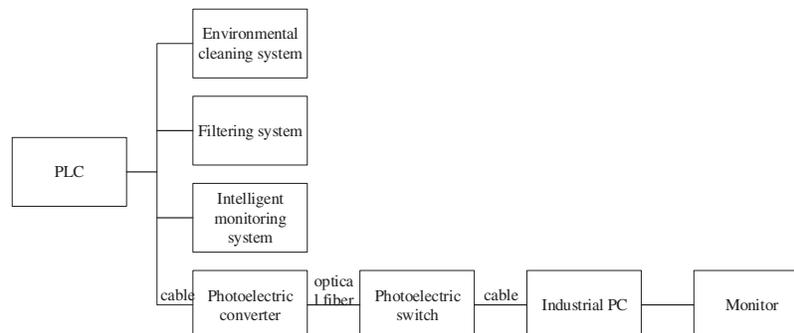
**Figure 1:** System wiring topology
