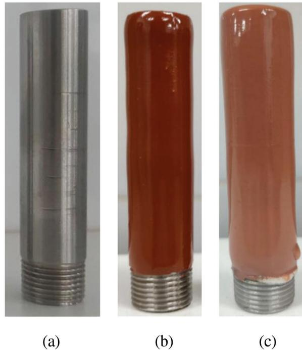
**Figure 2:** Image of a “cold” rod: a) Without a smooth coating; b) With a smooth coating No. 1; c) With a smooth coating No. 2
