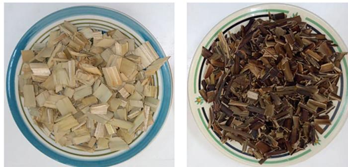
**Figure 4:** Typha aggregate (left untreated, right treated)
