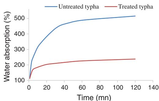
**Figure 6:** Absorption kinetics of aggregates
