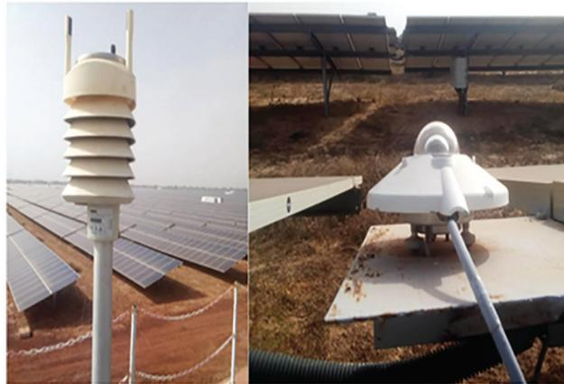
**Figure 2:** Weather station and irradiance sensors
