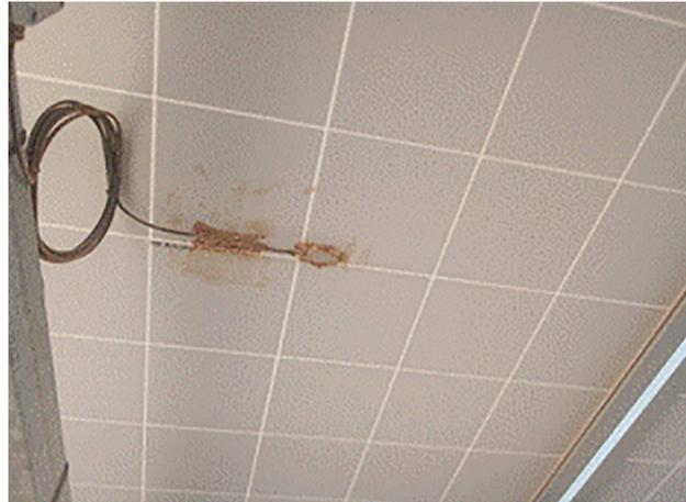
**Figure 1:** Temperature sensor mounted on the backside of module
