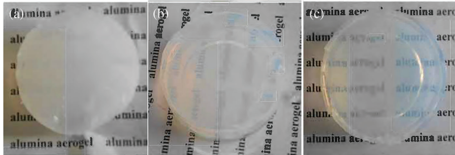
Figure 3: The effect of temperature on the gel; (a) 20°C, (b) 40°C, (c) 60°C
